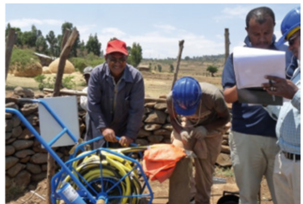
Figure 3. Field methods as conducted during Survey 2. Clockwise from top left; pump component inspections; pumping test - used to assess aquifer yield; field chemistry - used to assess corrosivity of water and overall water quality; borehole inspections - used to assess borehole construction.
