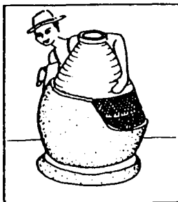
Applying the mortar layers
