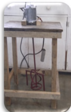
Figure 14 One of the two custom made mixers
