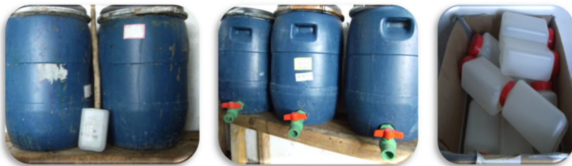
Figure 18: sludge sampler (left); drums used for gravitational settling (middle); collection jars (right)
