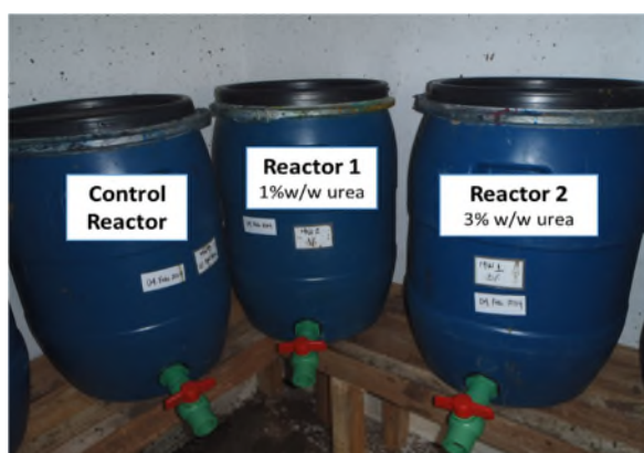
Figure 10: Urea Testing Field Set Up
