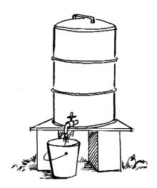
Next get some round stones, about 2-4 cm in diameter, and place them in the container around the opening where the tap has been put. Place the stones in such a way that the opening to the tap is not blocked off completely.
