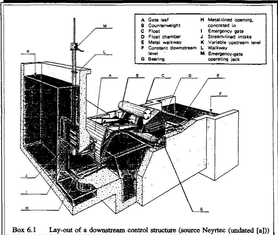
Box 6.1 Lay-out of a downstream control structure (source Neyrtec (undated [a]))
