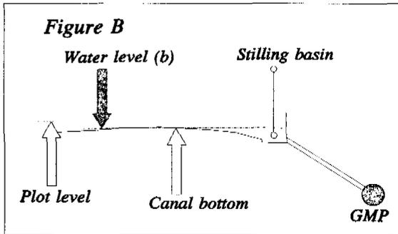
b) Situation some time after the GMP has been turned off: The water seems to have 'returned' from the plot to the lowest parts of the canal and the stilling basin.
