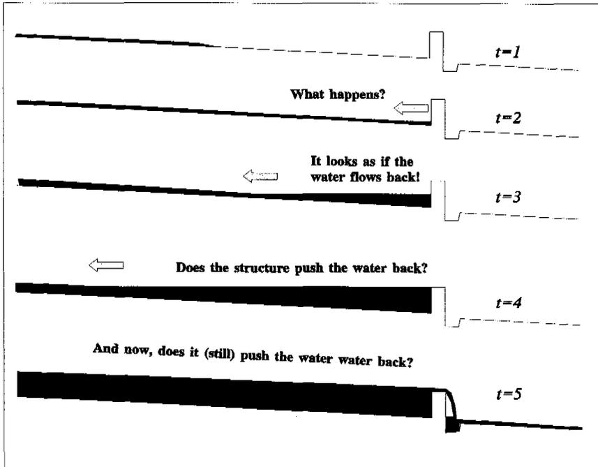
Later on, the water falls into an inverted siphon. When it reaches the other part of the road, the water rises in its downstream end. *Does the water flow upward?*
