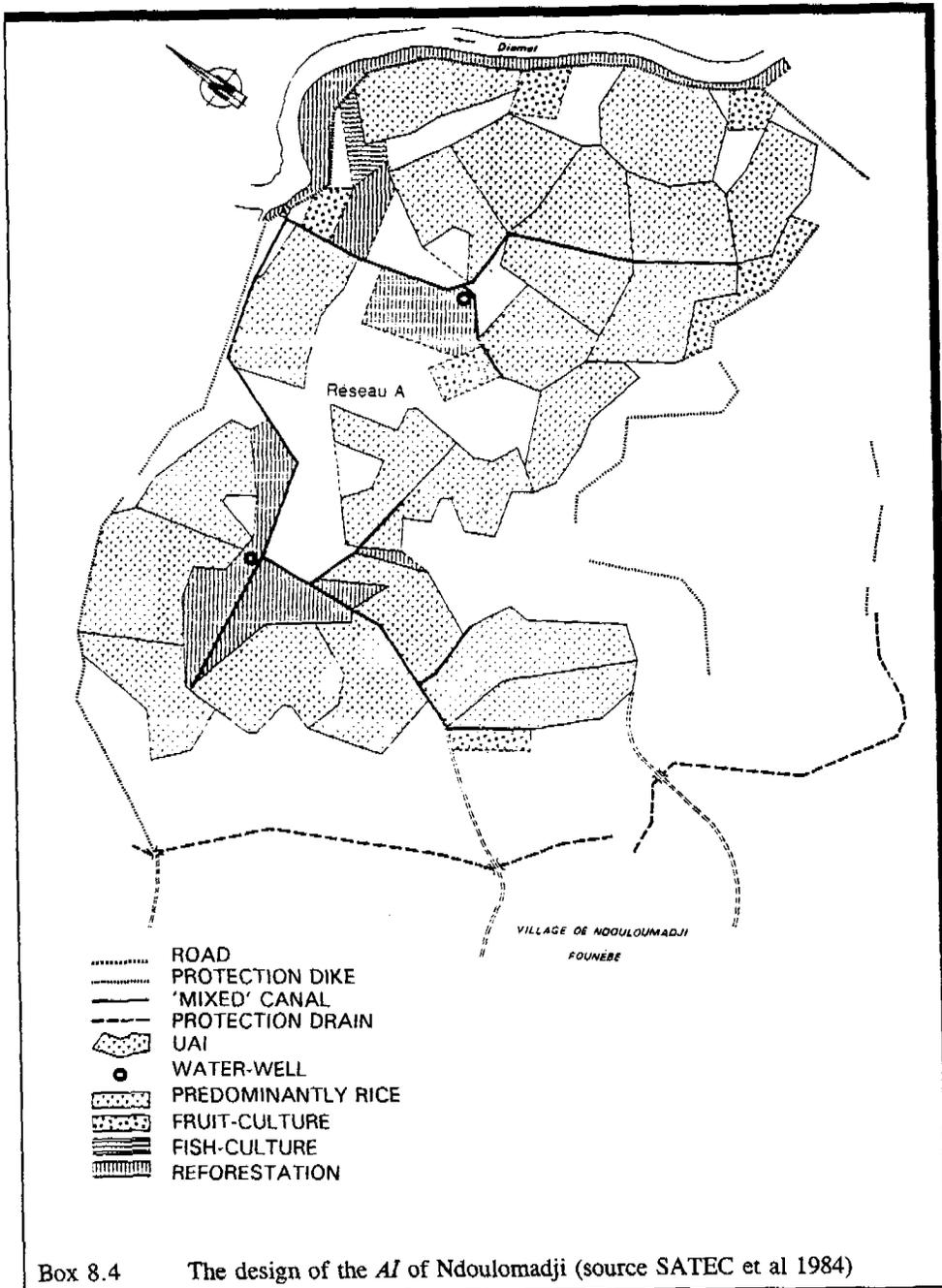
Box 8.4 The design of the AI of Ndoulomadji (source SATEC et al 1984)
