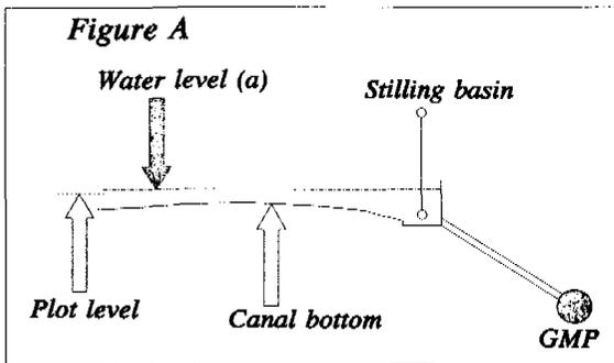
a) Situation during irrigation: the GMP is turned on and the water flows to the plot.
