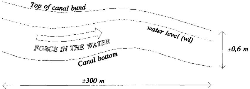
*Longitudinal section of a field canal (not to scale)*
