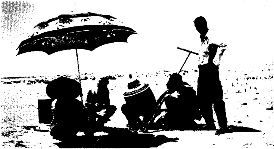
Sampling soil from different depths in Senegal using a simple hand auger. From the soil sample, moisture can be extracted and measured for the stable isotope and tritium contents.
