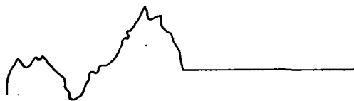
( d ) Float caught or slipping transmission
