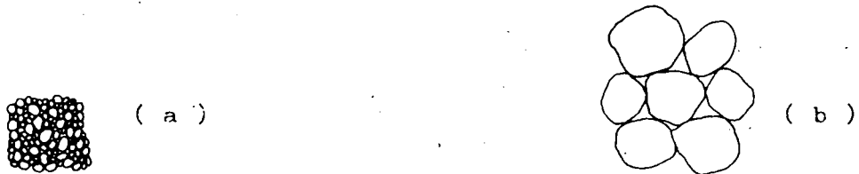
Fig. 2 Permeability in rocks : Impermeable rock-grains are so small and tightly packed that any water there may be is tightly held to the grains by adhesive forces, ( b ) permeable rock - water can move through larger spaces although some of it is held
