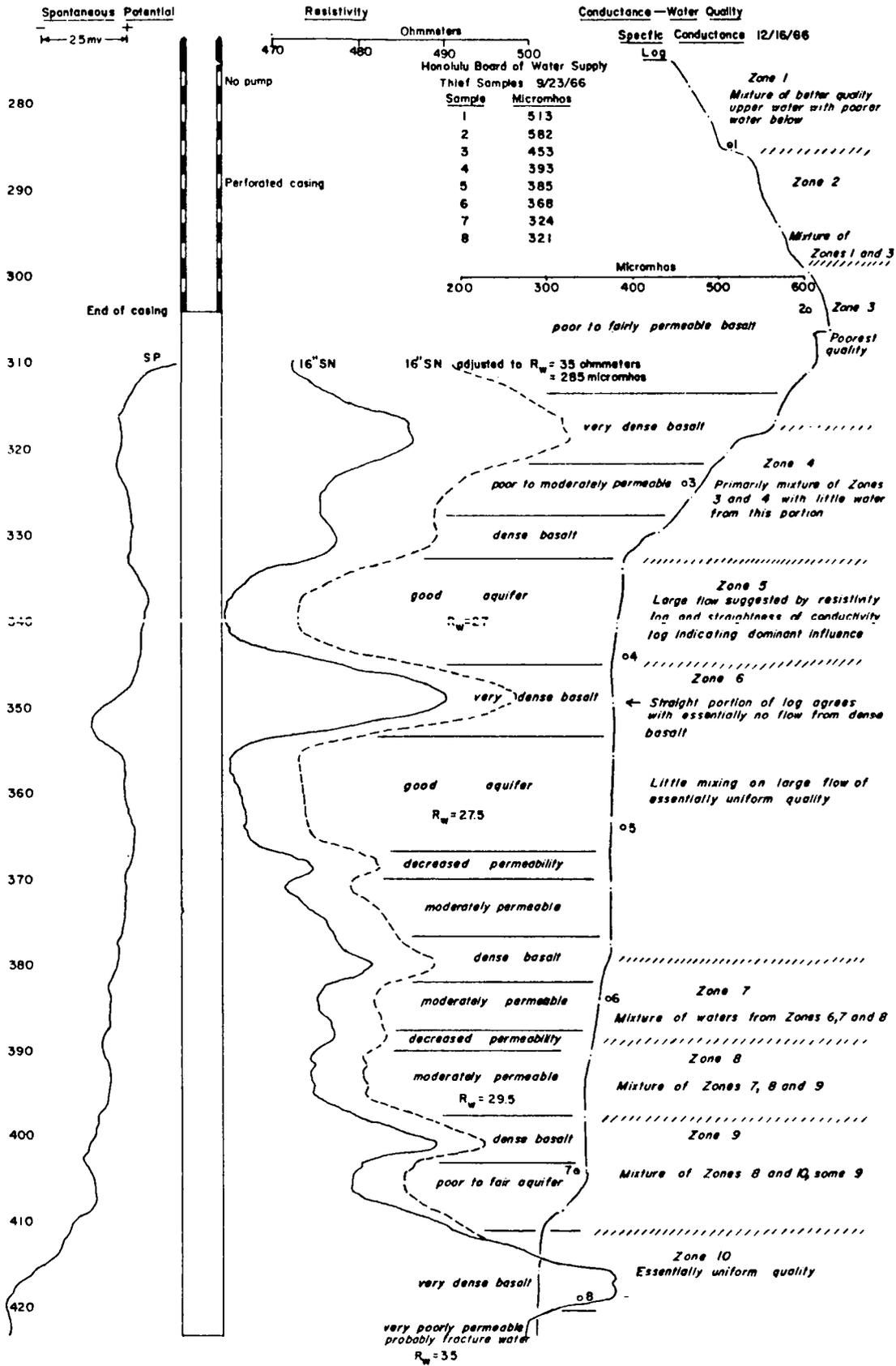
FIGURE 9. ELECTRIC WELL LOGS FOR WELL NO. 202-C, PEARL CITY, OAHU.
