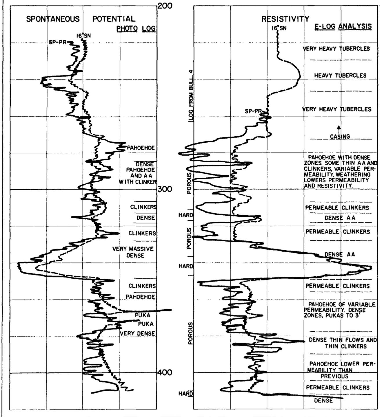
FIGURE 16. CORRELATION OF ELECTRIC LOGS, DRILLER'S LOGS AND PHOTO LOG OF WELL 128E, KALIHI, OAHU.
