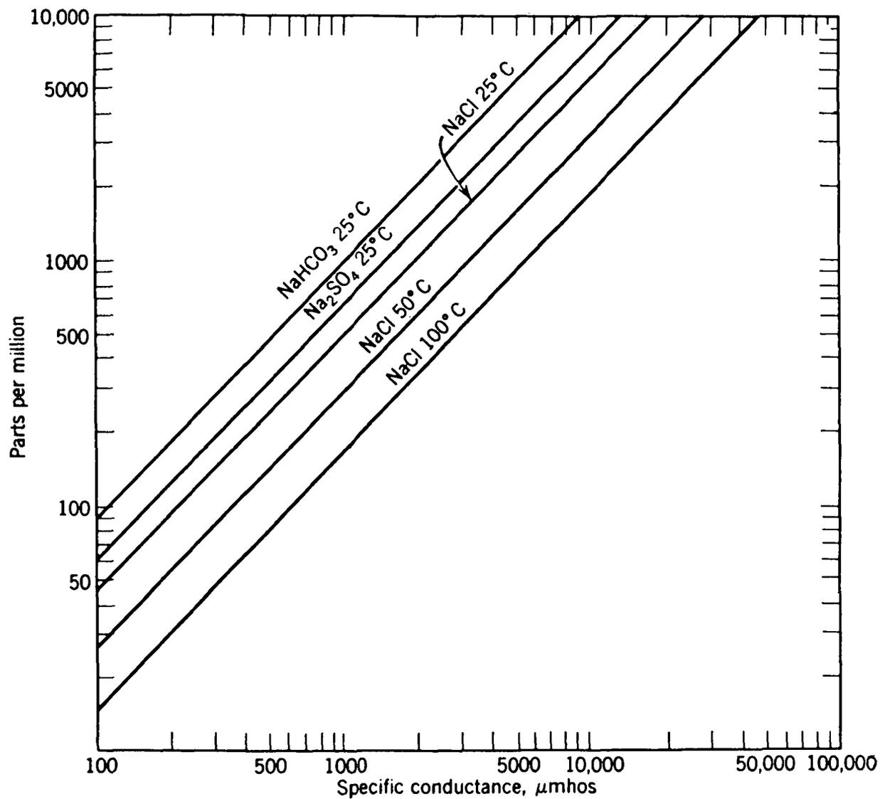
FIGURE 4. SALINITY, TEMPERATURE, AND CHEMICAL EFFECTS ON CONDUCTIVITY. (AFTER DAVIS AND DEWIEST, 1966).
