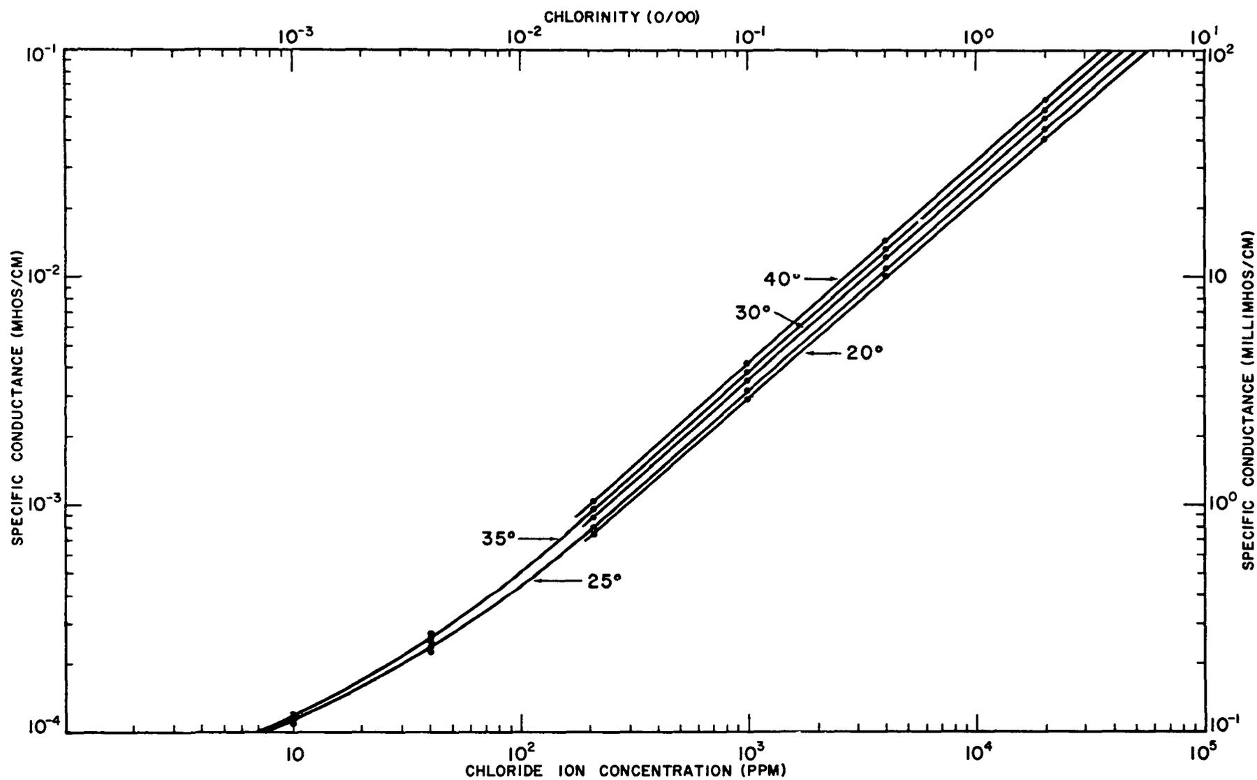
FIGURE 8. SALINITY VERSUS CONDUCTIVITY (AFTER COX, ET AL., 1969).
