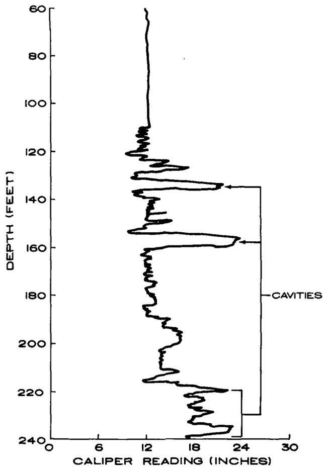
B. CALIPER LOG SHOWING CAVITIES IN KAIMUKI WELL 7A.
