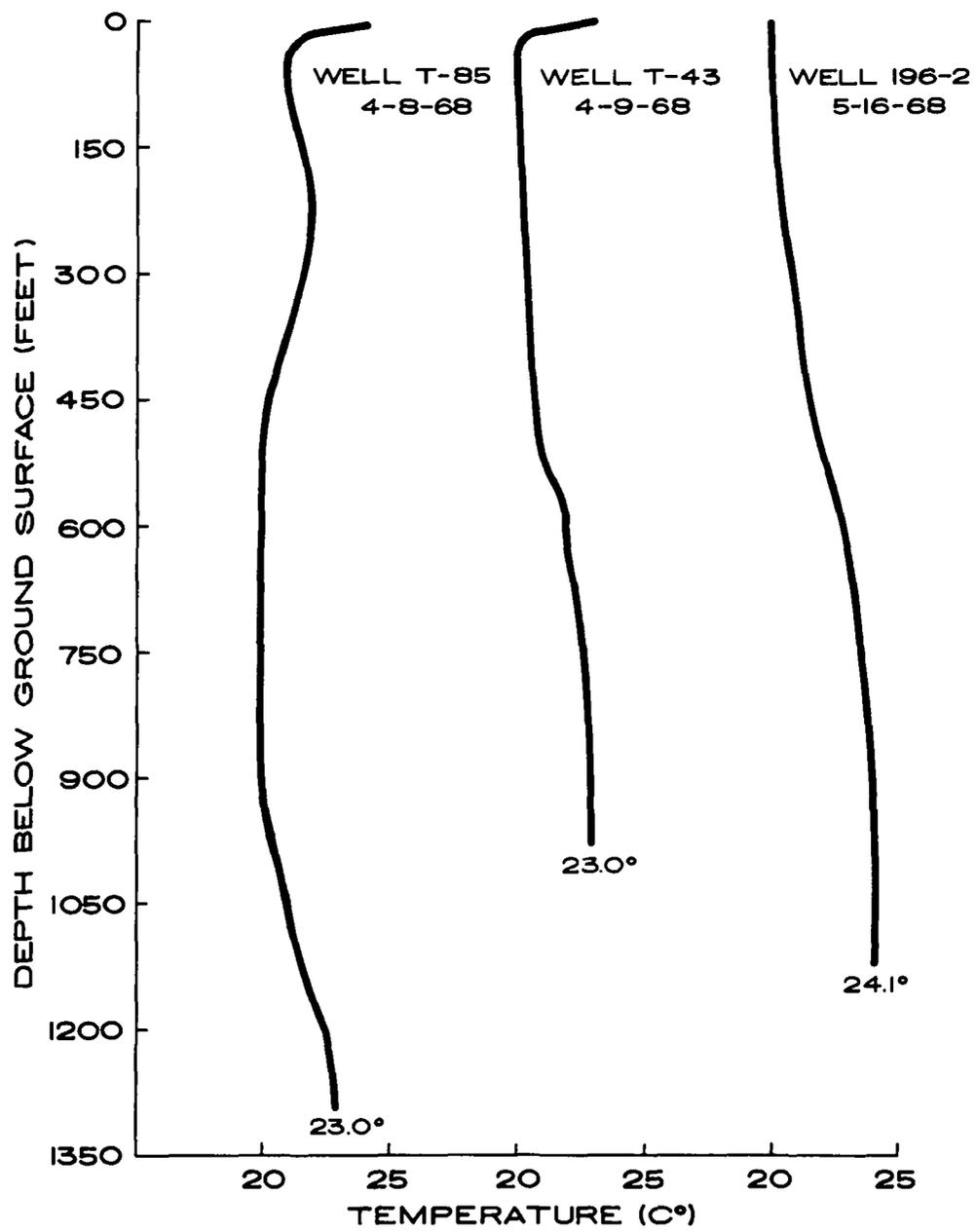
FIGURE 7. TEMPERATURE LOGS FOR WELLS T-85 (BERETANIA), T-143 (PUNALUU), AND 196-2 (PUNANANI).
