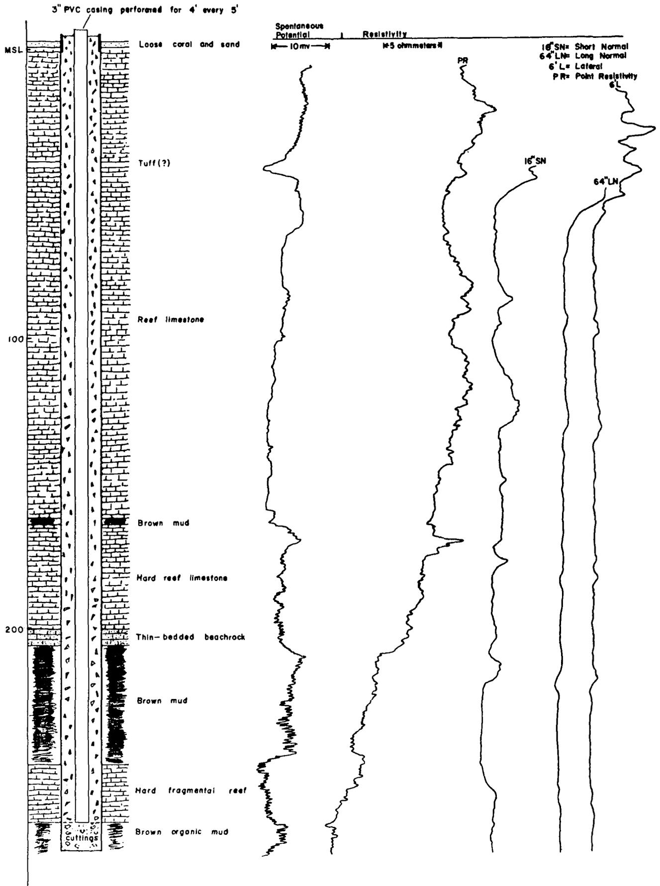
FIGURE 11. ELECTRIC LOGS AND GEOLOGIC LOG FROM WELL NO. T-133-1, EWA BEACH, OAHU.
