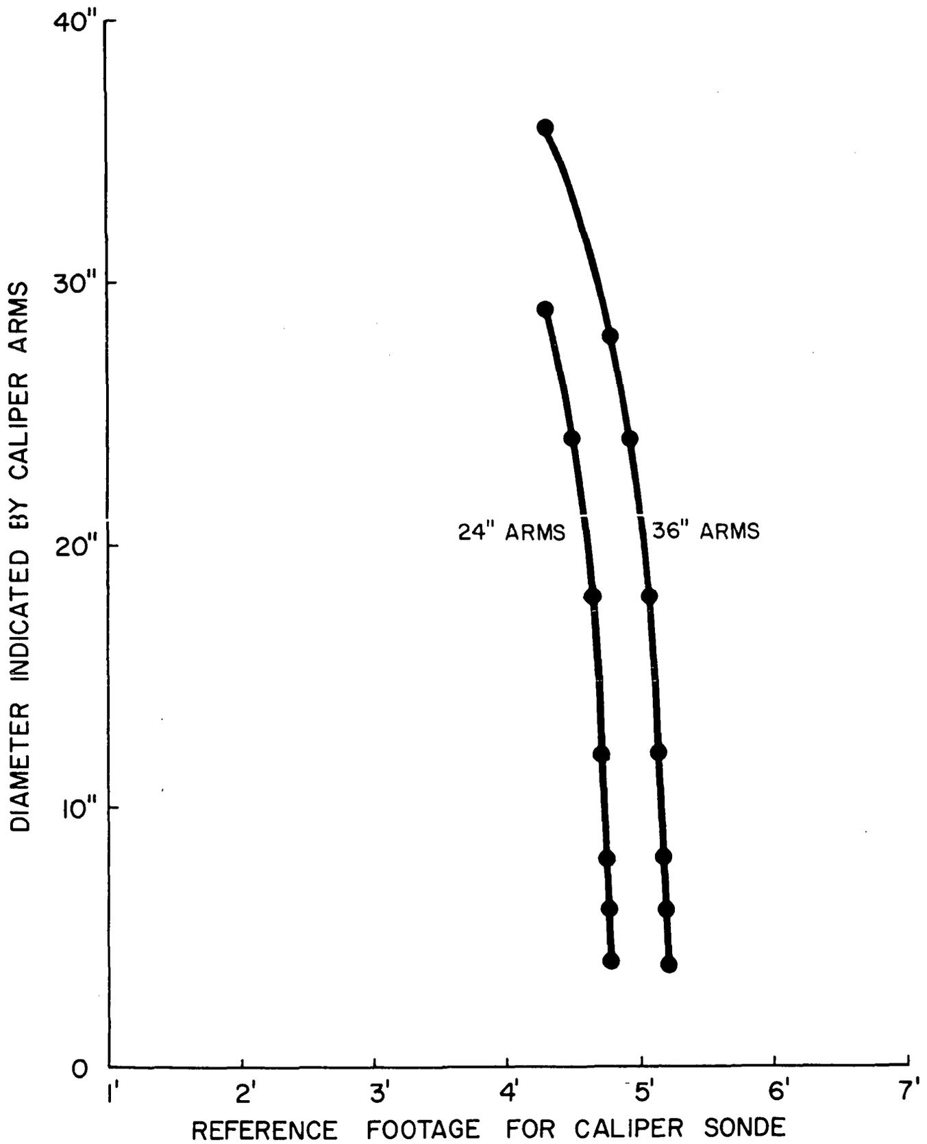
FIGURE 5. CORRECTION CURVE FOR CALIPER REFERENCE FOOTAGE.
