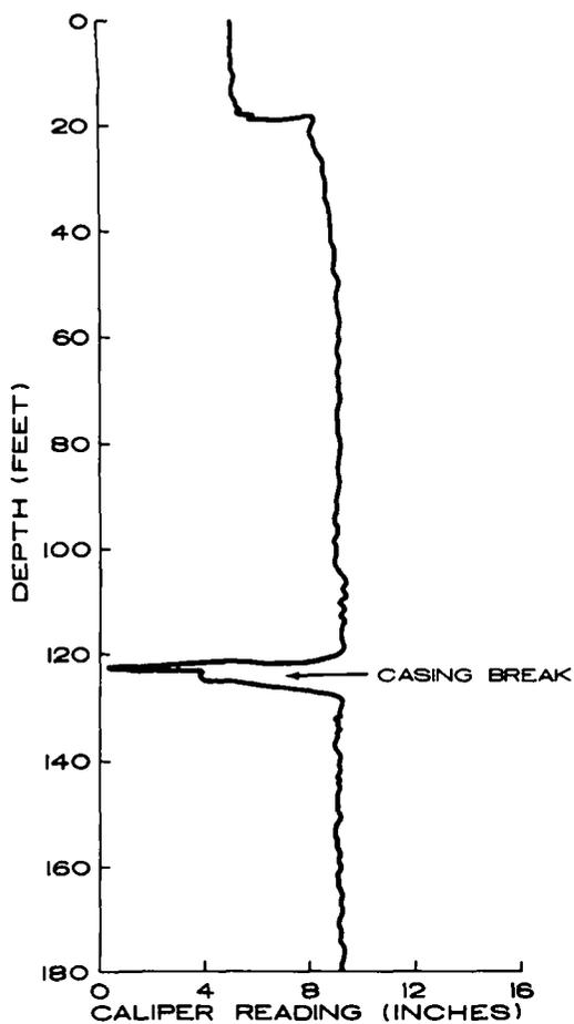
A. CALIPER LOG SHOWING CASING BREAK IN BERETANIA WELL 88-B.
