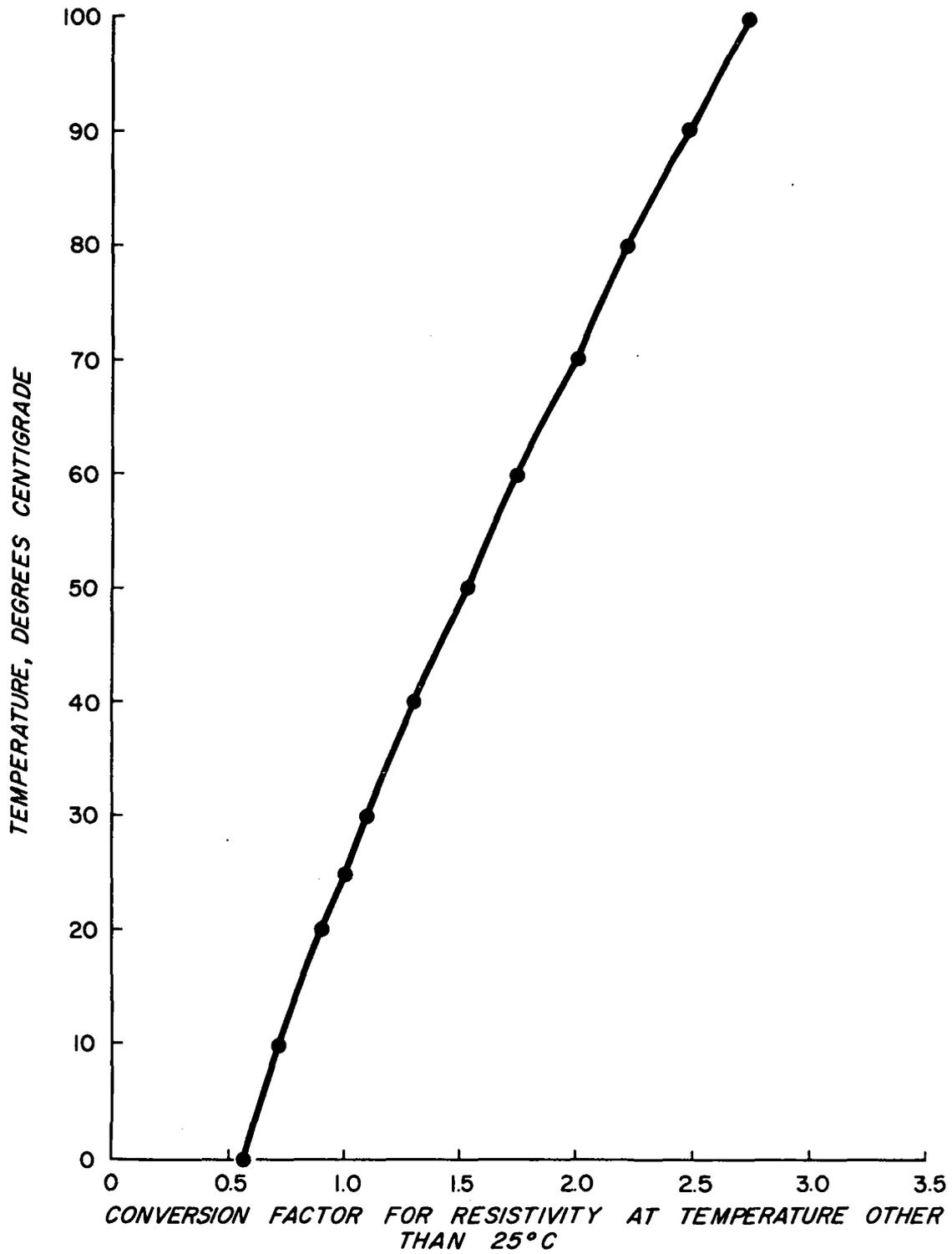
FIGURE 13. CURVE FOR ADJUSTING RESISTIVITY TO 25°C.
