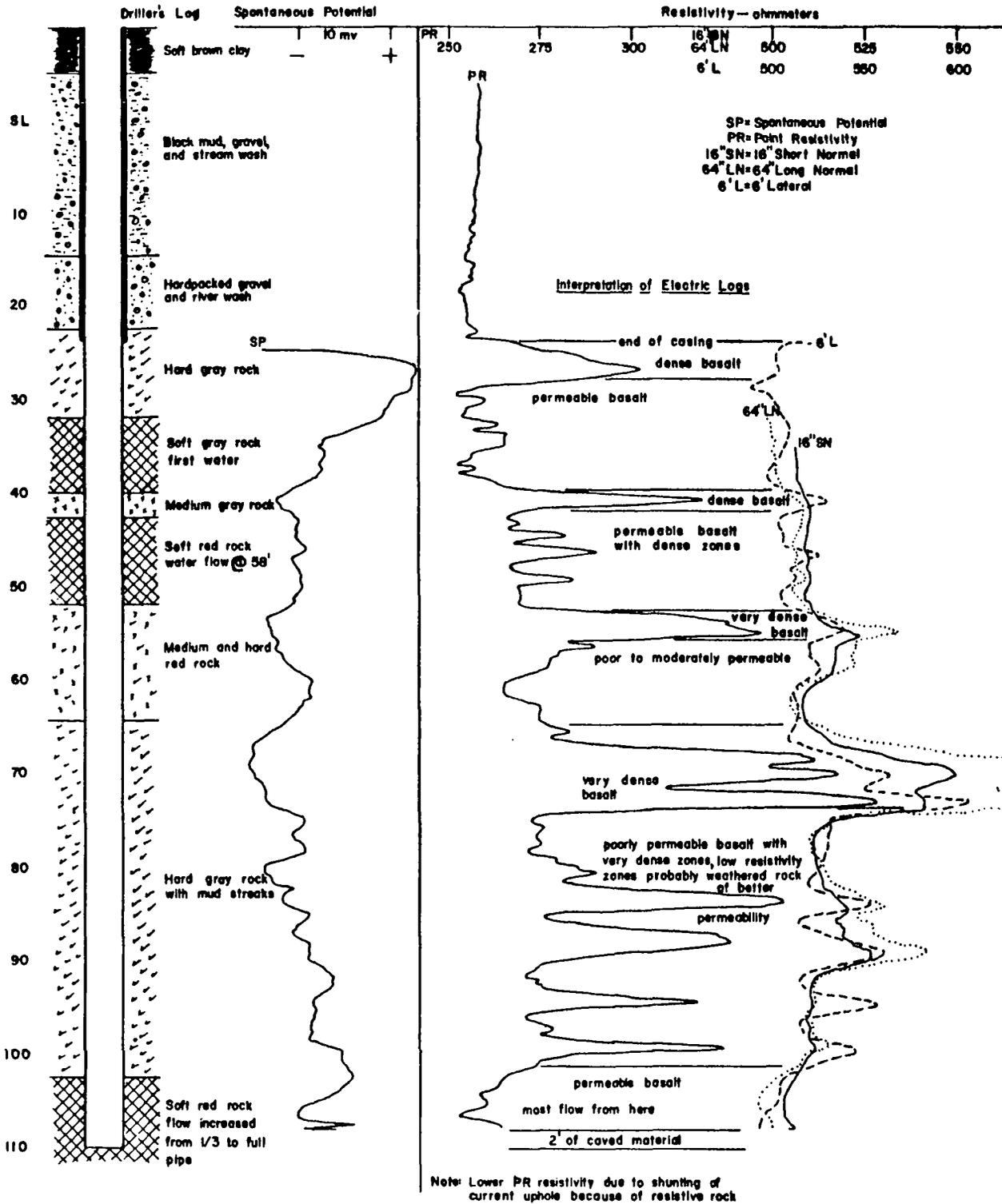
FIGURE 12. ELECTRIC LOGS AND GEOLOGIC LOG FROM WELL NO. 200-4, PEARL CITY, OAHU.
