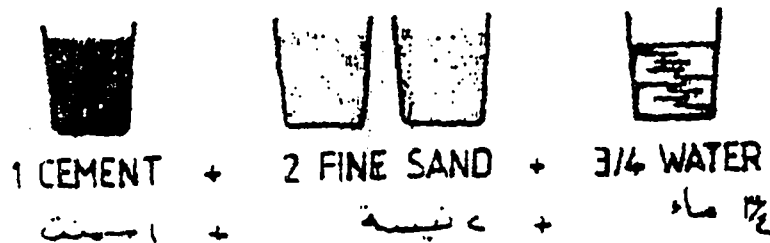
Diagram 16 - Design Mix for Mortar in Ferrocement Tank.
