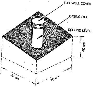
COVER TUBE WELL CASING PIPE DIG A SQUARE PIT 75 CM BY 76 CM AROUND CASING PIPE AND 40 CM DEEP FROM GROUND LEVEL
