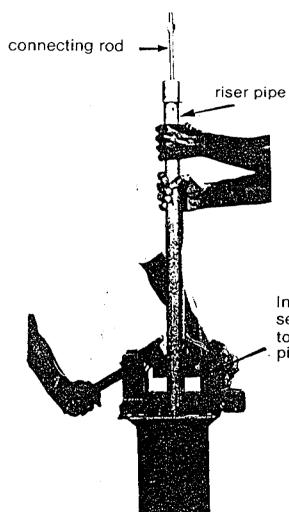
Insert the self locking clamp to clamp the riser pipe as shown.
