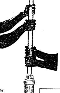
Lower cylinder, first pipe and connecting rod into tube well.
