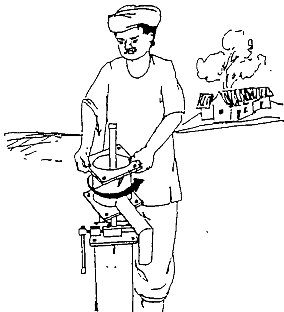
FIG:4.12 : REMOVE WATER TANK
