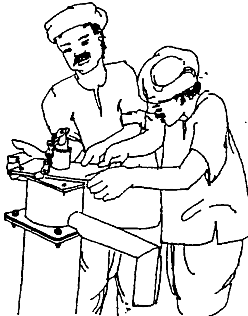
FIG:4.41 PUTTING MIDDLE FLANGE OVER WATER TANK
