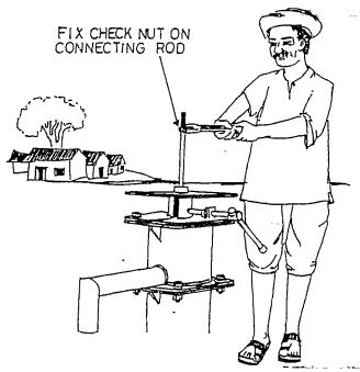
FIG:4.38 TIGHTENING CHECK NUT
