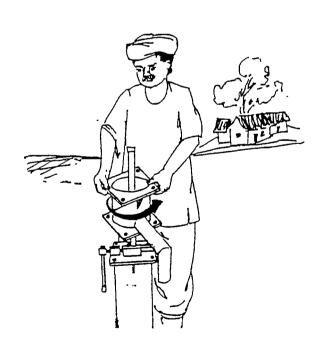
FIG:4.12 : REMOVE WATER TANK
