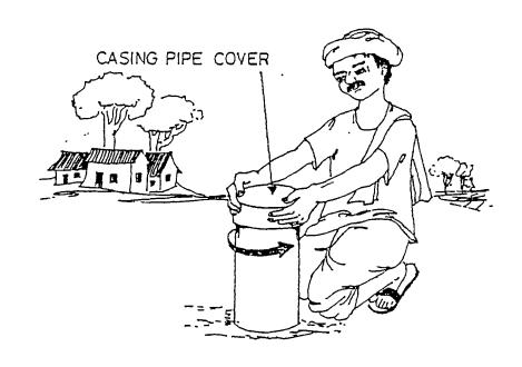
FIG: 4222 REMOVE COVER OF CASING PIPE
