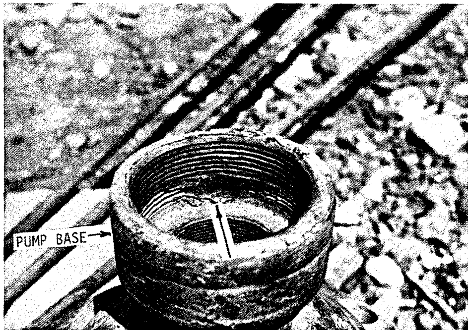
Arrow shows plaster placed by manufacturer to cover porosity. Pump was accepted and installed as shown.
