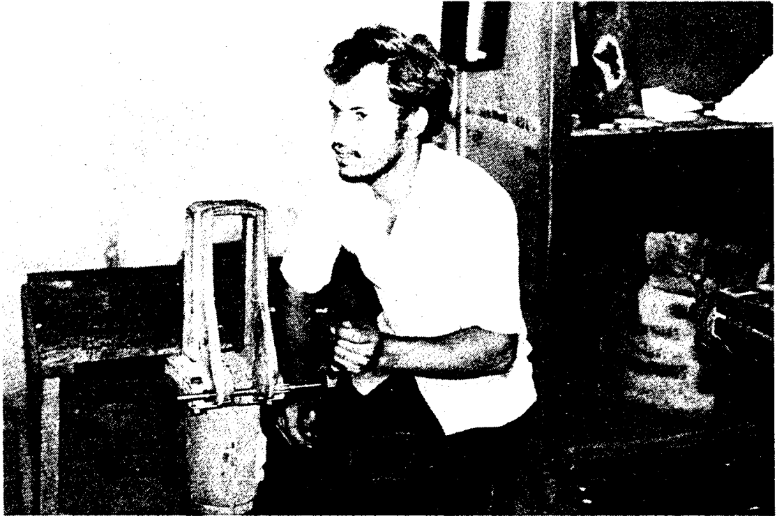
CAP REAMING TO CORRECT MISALINGED DRILLED HOLES
