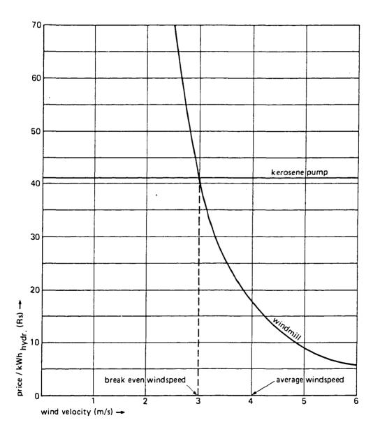
One can see that the break-even wind speed is below the actual average wind speed, indicating that the windmill can pump water at a lower cost than a kerosene pump.
