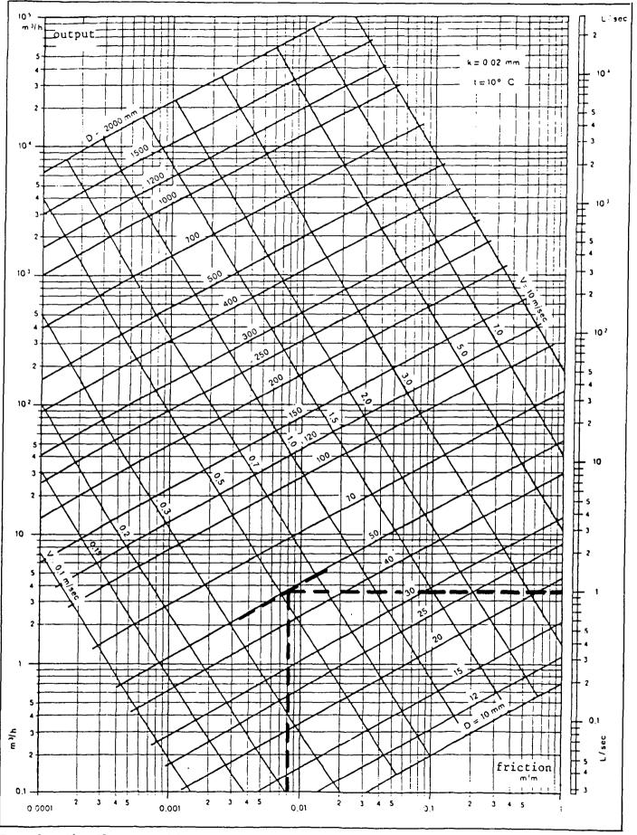
APPENDIX III FRICTION LOSSES IN PVC AND PE PIPES (m head loss/m pipe)
