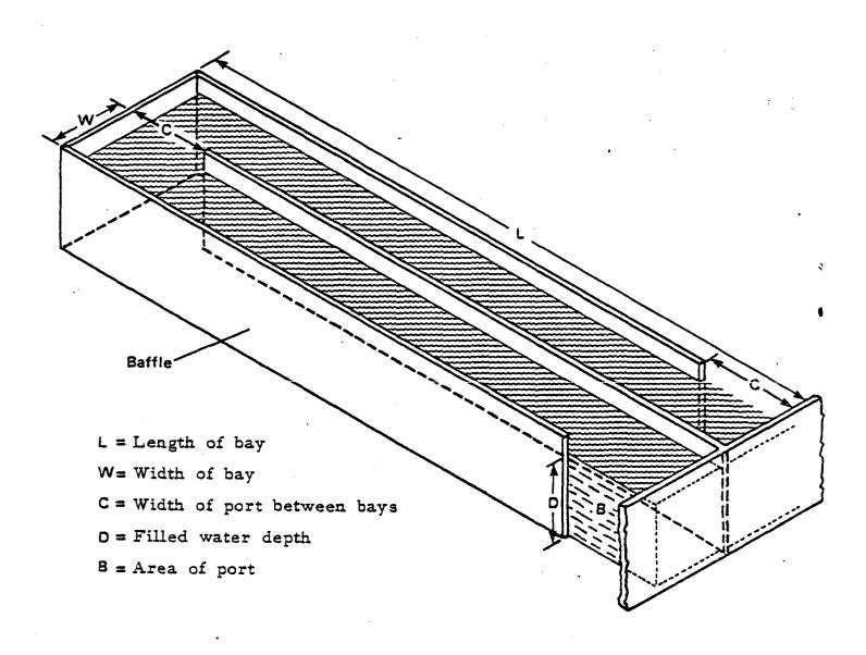
Figure 1. Diagram of a baffle arrangement in a serpentine channel
