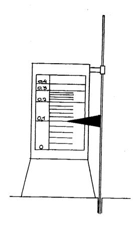
Once or twice a day, the filtration rate should be checked by looking at the position of the pointer on the scale.
