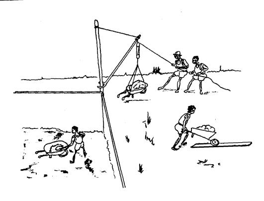
Remove the sand from the filter or the first strip and place it on a clean area beside the filter. Take care not to disturb the layer of gravel. The sand can be thrown out of the filter or carried out in a wheel barrow and a gantry. Instead of removing the sand from the filters, sand from the first strip can be stored temporarily at the opposite end of the filter box.
