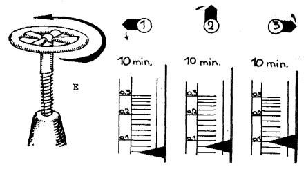
Turn valve (E) counterclockwise to increase the filtration rate.
