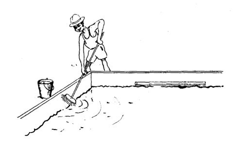
Brush the walls and continue to discharge water through the overflow until all floating dirt is removed. Step 3: drain the water from the filter.
