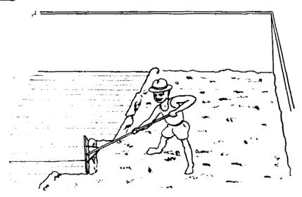
Be careful not to pollute the sand, therefore do not enter the filter box with dirty shoes, and clean the levelling tool beforehand.
