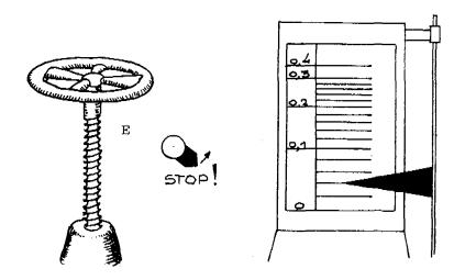
The resistance of filter skin gradually increases. When it becomes too high, that is when valve E is fully open and the filtration rate cannot be maintained, the filter needs to be cleaned.
