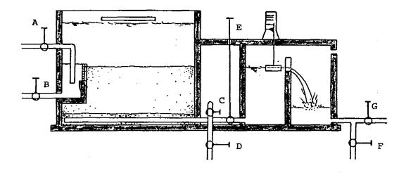
Step 6: increase filtration rate every half hour by 0.02 m/h and continue until design flow is reached.
