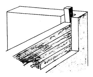
If necessary, adjust the inlet box to the new sand level. The height of the timbers should be just a little over the level of sand in the filter, so that the supernatant water can be drained without washing out filter sand. When the timbers have been adjusted, the upper timber needs to be pinned in place to prevent it floating away.
