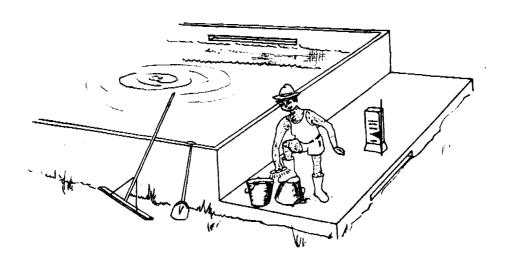
Dirt on equipment or on boots may be carried into the filter unit and be pressed into the filter bed. This will contaminate the filtered water after re-starting the filtration process, or will require the removal of a thicker layer.
