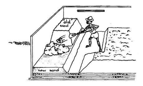
Replace the sand, which contains many micro-organisms, on top of the new sand. Here the advantage of working in strips for large units becomes obvious. The "old" sand in the second strip can be removed and placed directly on top of the "new" sand in the first strip, and the "old" sand in the third strip onto the second and so on.
