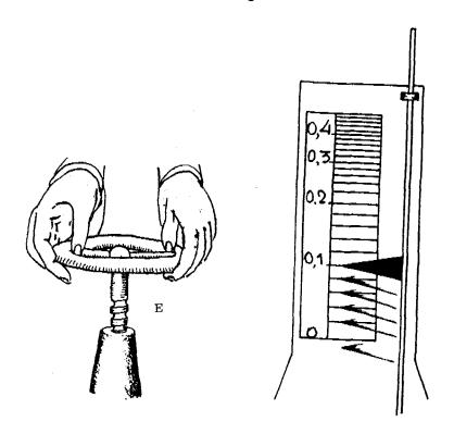
The filtration rate needs to be increased gradually to facilitate the initial removal of impurities from the raw water. When adjusting the rate it must be remembered that it will take at least five minutes before the flow indicator shows the new rate of filtration.
