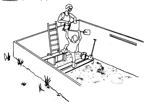
Step 4: mark out areas of about 3x3 m by scraping narrow strips, and place boards on these strips.
