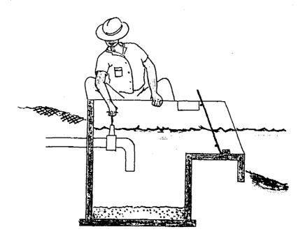
When the river water becomes very turbid, the filters clog up rapidly and frequent cleaning will be required. Therefore, it may be useful to stop the intake of raw water temporarily in periods of excessive turbidity, such as during the monsoon.
