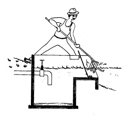
If the screen is not cleaned daily, the intake may become blocked, too little water will flow to the plant and the pumps may run dry and become damaged.
