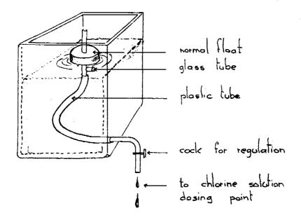
A drip chlorinator is often used for dosing the chlorine solution.
