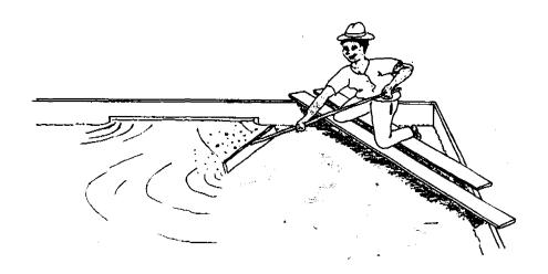
Scum floating on the surface of the water and filamentous algae must be removed because this may interfere with the purification process. To remove this material:
