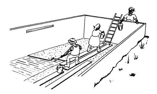
Usually the scrapings cannot be thrown over the side of the filter. They must be loaded into some type of bucket which can be used to carry or lift the scrapings out of the filter bed to the sand washing area.
