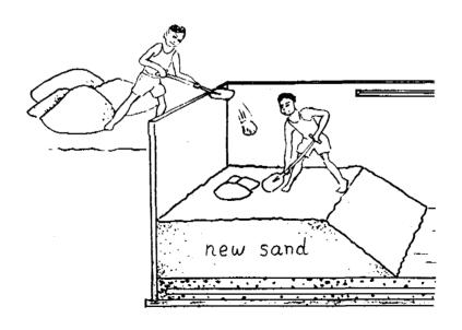
Place the washed and cleaned new sand in the emptied filter or on a strip on top of the gravel layer from which the sand has been removed. Usually, only about 30 cm has to be placed, because the "old" sand layer of 50 cm will be replaced on top.
