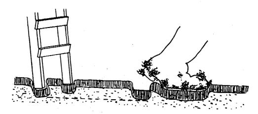
If boards are not placed on the sand, workers entering the filter unit will press the filter skin into the sand bed. This will make scraping much more difficult because a much thicker layer will have to be removed.
