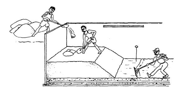
Throw clean sand in the filter and spread it evenly on top of the gravel to a depth of at least 80 cm.
