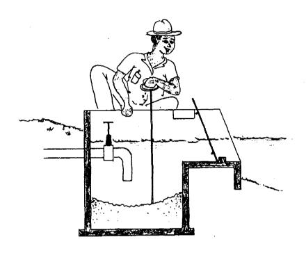
Sand and silt will settle in the sump. Each time the sump is visited, the level of the deposit in the sump should be checked with a measuring stick.
