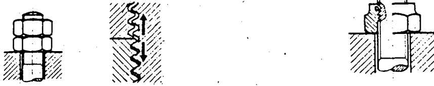
Fig. 46.1 Locking arrangements in which forces act on the threads (e)
