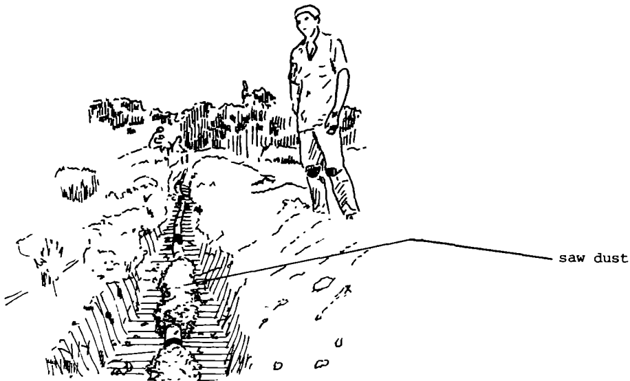
figure 22. Bamboo testline with CCA treated saw dust envelope
