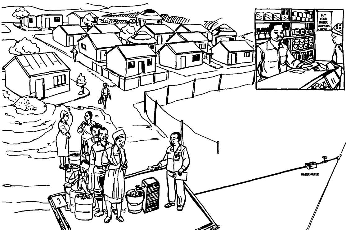
Figure 2.2 RDP basic level of service: Cost recovery option no. 2: Public standpipe: Prepaid with attendant
