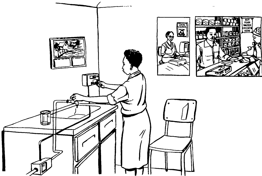
Figure 2.11 Highest level of service: Cost recovery option no. 3: Household connection: Prepaid electronic vending
