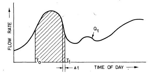
$\int_{T_{O}}^{T_{I}} Q_{t} dt = G = \text{shaded area of graph}$
