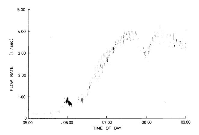
Fig. 13(b). Predicted flow into area 2 excluding kitchen tap use - European plumbing system
