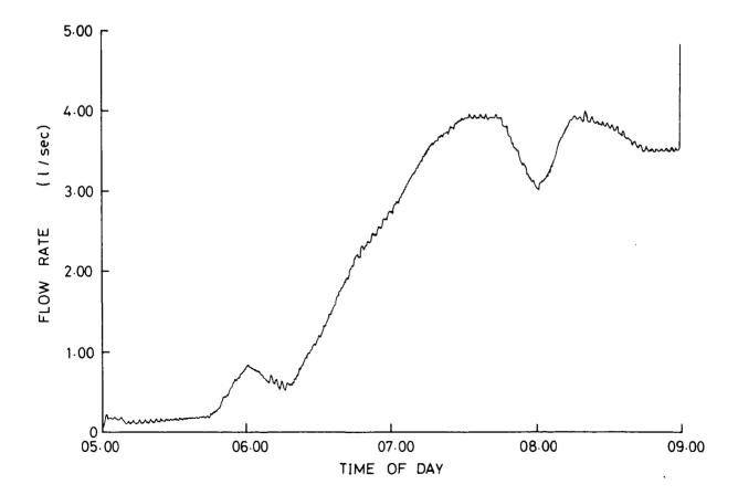
Fig. 10(b). Simulation of flow into area 2 excluding kitchen tap use
