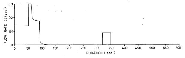
Fig. 11. Calculated flow through service pipe for plumbing system with no storage (calculated for the use sequence shown in Fig. 4)
