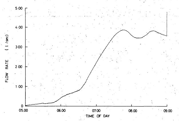
Fig. 20(b). Predicted flow into area 2 – tank inflow rate restricted to 0.01 litres/sec – excluding kitchen tap use (assuming 10% of the uses have a second use starting 15 minutes after the first)
