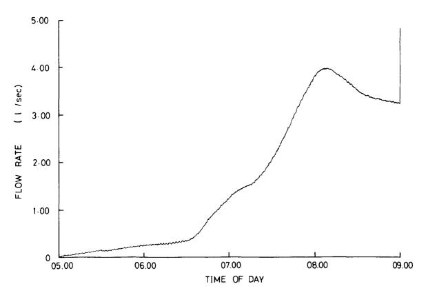
Fig. 19(b). Predicted flow into area 1 – tank inflow rate restricted to 0.01 litres/sec – excluding kitchen tap use (assuming 10% of the uses have a second use starting 15 minutes after the first)
