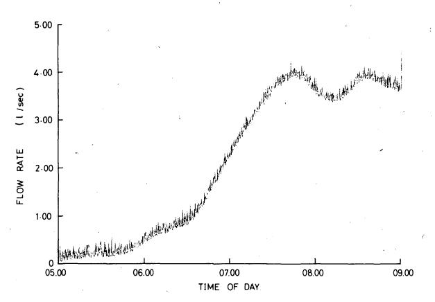
Fig. 18(a). Predicted flow into area 2 with tank inflow rate restricted to 0.01 litres/sec (assuming the start of water uses within a single house are at least 30 minutes apart)
