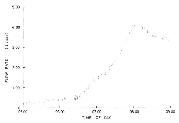
Fig. 19(a) Predicted flow into area 1 – tank inflow rate restricted to 0.01 litres/sec (assuming 10% of the uses have a second use starting 15 minutes after the first)
