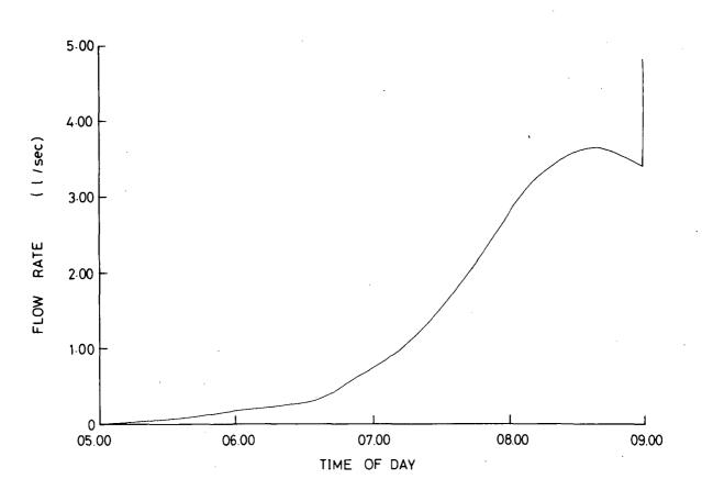
Fig. 24(b). Storage tank emptying/refilling cycle, excluding kitchen tap use. Predicted flow into area 1 - filling time 60 minutes
