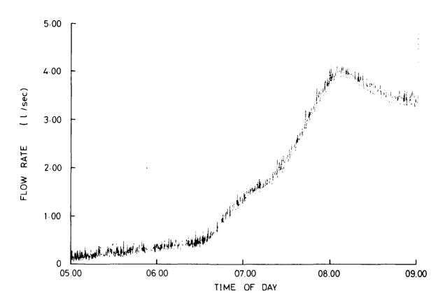
Fig. 17(a). Predicted flow into area 1 with tank inflow rate restricted to 0.01 litres/sec (assuming the start of water uses within a single house are at least 30 minutes apart)
