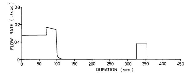
Fig. 14. Calculated flow using modified use sequence
