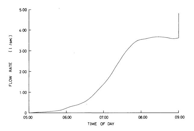
Fig. 25(b). Storage tank emptying/refilling cycle, excluding kitchen tap use. Predicted flow into area 2 - filling time 60 minutes
