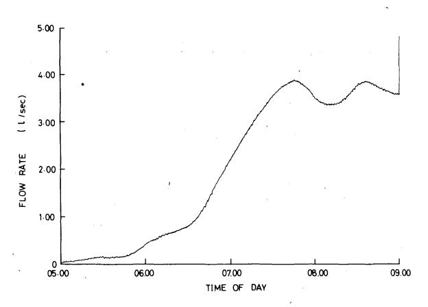
Fig. 18(b). Predicted flow into area 2 with tank inflow rate restricted to 0.01 litres/sec excluding kitchen tap use (assuming start of water uses within a single house are at least 30 minutes apart)
