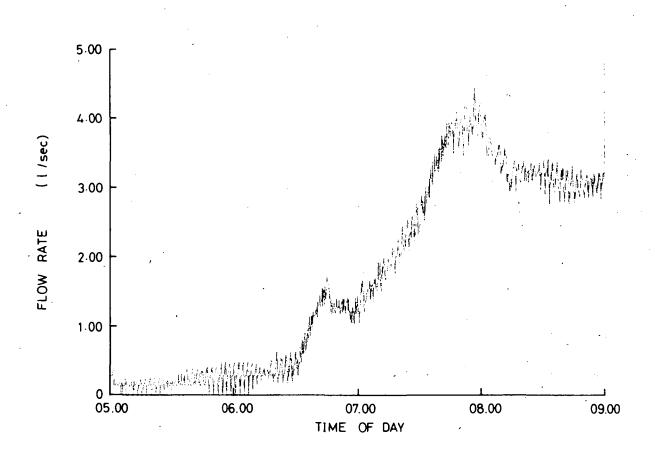
Fig. 15. Predicted flow into area 1 using modified use sequence shown in Fig. 11 and excluding kitchen tap use
