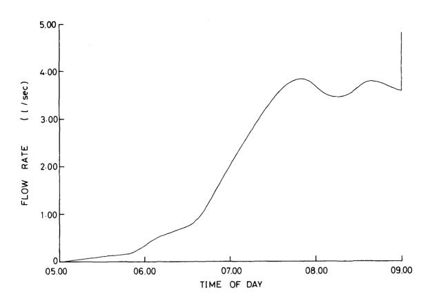
Fig. 23(b). Storage tank emptying/refilling cycle, excluding kitchen tap use. Predicted flow into area 2 - filling time 30 minutes
