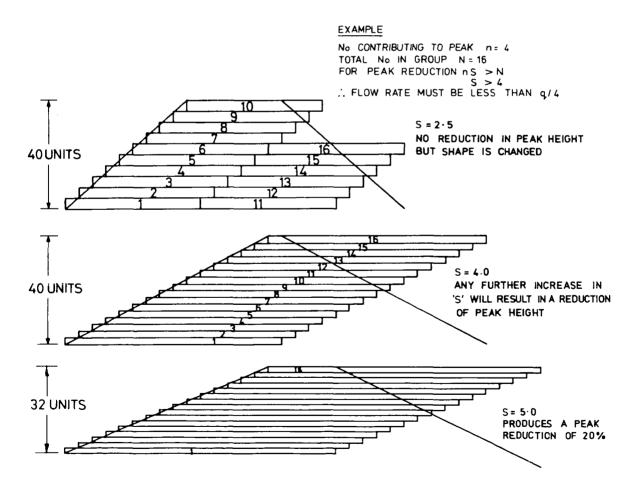
Fig. 27. Effect of restricting tank inflow rate
