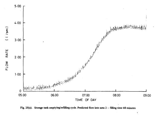
Fig. 25(a). Storage tank emptying/refilling cycle. Predicted flow into area 2 - filling time 60 minutes
