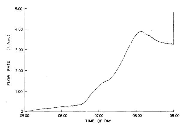
Fig. 17(b). Predicted flow into area 1 with tank inflow rate restricted to 0.01 litres/sec excluding kitchen tap use (assuming start of water uses within a single house are at least 30 minutes apart)
