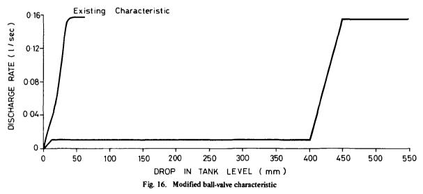
If the storage tank in any house fills at a rate of 0.01 litre/sec, the filling time for the use shown in Fig. 4 will be approximately 30 minutes. If an individual with this particular use sequence occupies the bathroom for, say, 15 minutes, then it is possible that a second person could use water within the house before the tank had refilled from the first use. Under these circumstances the flow through the distribution pipe would not increase to 0.02 litre/sec, but would remain at 0.01
