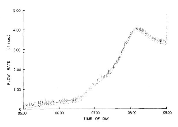
Fig. 22(a). Storage tank emptying/refilling cycle, Predicted flow into area 1 - filling time 30 minutes
