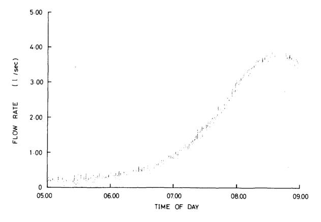
Fig. 24(a). Storage tank emptying/refilling cycle. Predicted flow into area 1 - filling time 60 minutes
