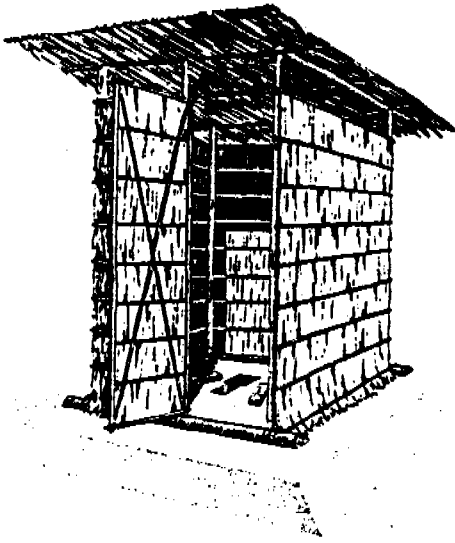
E. Palm-thatch wall and roof covering
