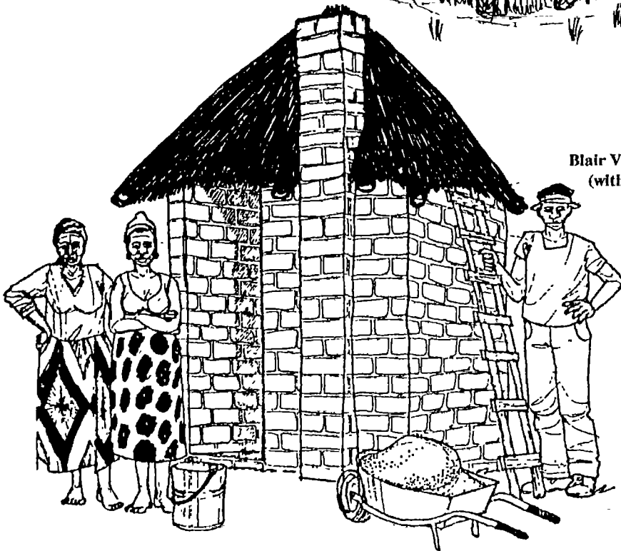
Blair VIP using 3 bags of cement (with grass roof)
