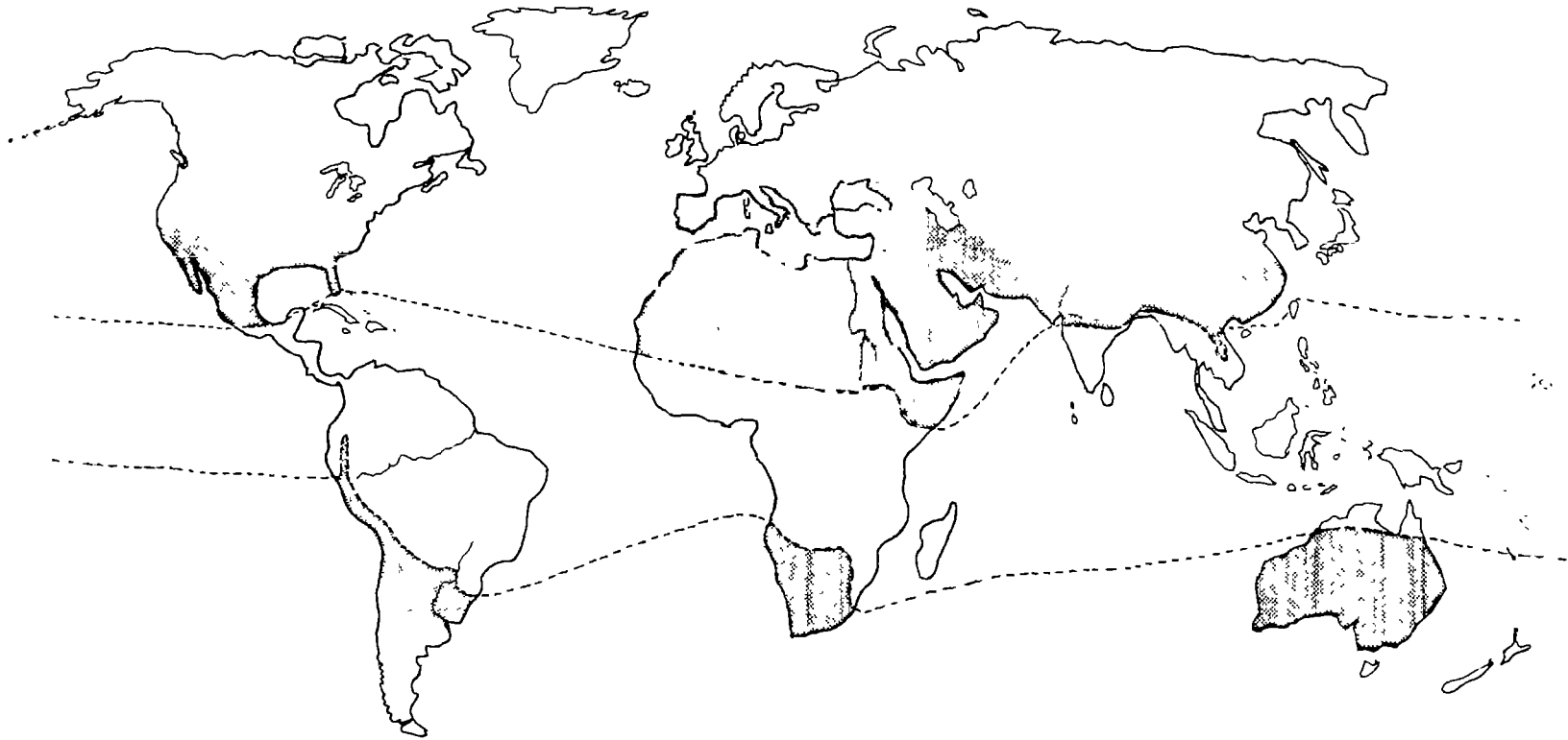
Figure 1.4 World climatic zones based on climate map in the Time atlas of the World. Anaerobic sewage treatment is definitely possible in the equatorial zone within the striped lines because of generally high ambient (sewage) temperature. Anaerobic sewage treatment is probably feasible in the grey-shaded areas (usually a sufficiently elevated sewage temperature). In white areas it may usually prove too expensive compared with other treatment methods.
