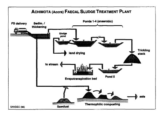
The Achimota FSTP treatment plant is in operation since 1990. Usually, a mixture of public toilet sludge and septage is treated at this site.
