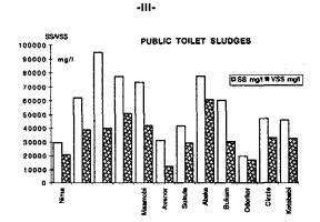
The variation of the SS/VSS concentrations in public toilet sludges from different parts of Accra/Ghana reflects the influence of the public toilet operation modus (frequency of emptying, groundwater or surface water intrusion)
