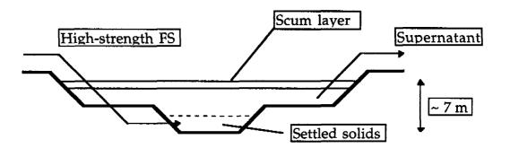
Deep anaerobic ponds are likely to constitute the simplest option; the removal of the separated solids may, however, prove to be difficult due to the depth of the pond. The presumably high density of the settled solids may preclude gravity draw-off under hydrostatic pressure.
