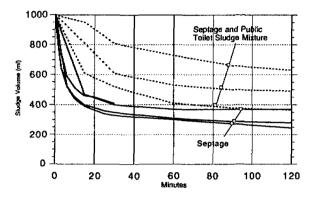
The mixture of septage and public toilet sludge shows poor settleability. The extent of this depends on the share of public toilet sludge and its degree of stabilization or digestion.
