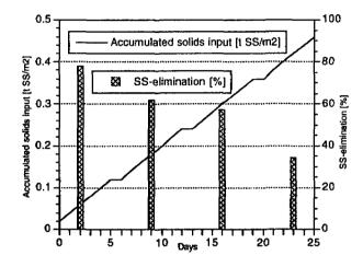
This Figure shows cumulative solids loading and suspended solids (SS) removal plotted as a function of tank operating time as observed at the Achimota FSTP.
