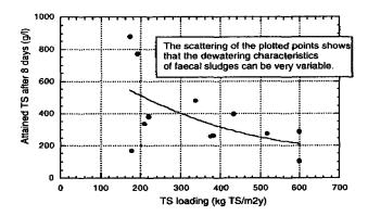
The figure shows the TS concentrations attained after a period of eight days as a function of TS loading rate. The experiments this figure is based on were conducted during the dry season with sludge application depths of  $\leq$  20 cm. Average temperature and period of sunshine, including pan evaporation, amounted to 27 °C, 7.8 hours/day and 5.4 mm/day, respectively.
