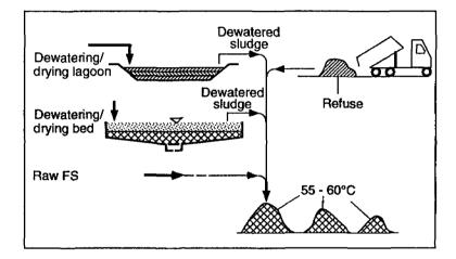
Example for co-composting solid waste and faecal sludge from bucket latrines :
