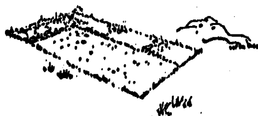
1 shallow excavation - level base
