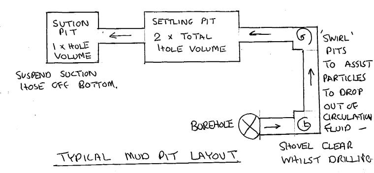
Bearing in mind the need to obtain the crucial up-hole velocity rate enough to lift but not erode the hole it would be useful to introduce a weir or flume to measure the flow of the returning circulation — adjusting pump valve or throttle setting to maintain a constant flow (see RIG MODIFICATIONS)
