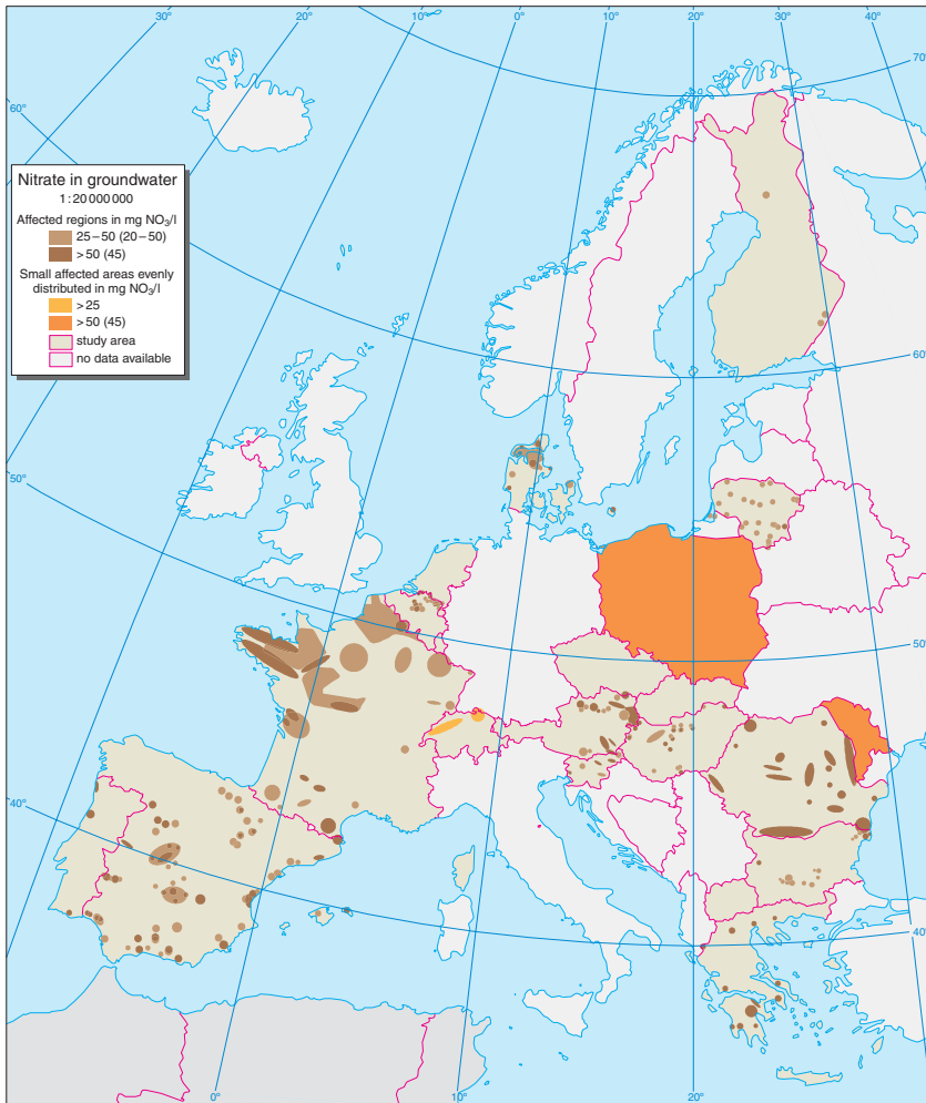
Fig. 2.10. Regions in selected countries in Europe affected by high nitrate concentrations in groundwater
