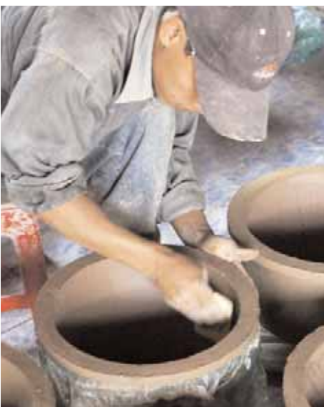
Inspection and smoothing of newly pressed filter pots
