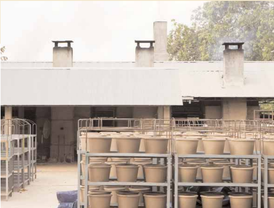
Filters ready for firing at the RDI factory in Kandal
