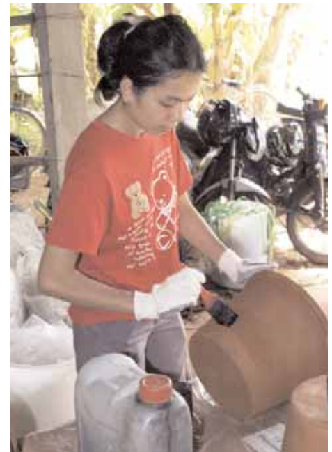
Impregnating the filters with silver nitrate improves bacterial removal
