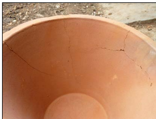
Figure 6-23: Firing/Cooling Crack (Pelita 2009)
