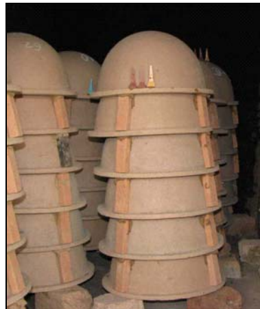
Figure 6-17: Filters Stacked for Firing, Myanmar (Thirst-Aid 2009)
