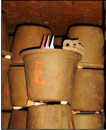
Figure 6-10: Draw Trials and Cones in Stacked Kiln (Cohen 2010a)
