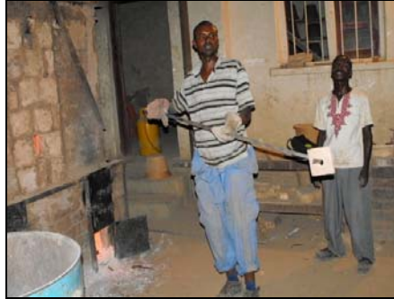
Figure 6-11: Draw Trial Being Removed (Cohen 2010a)
