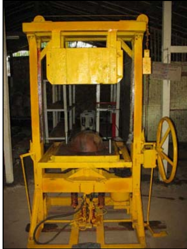
Figure 5-5: Filter Press with Wooden Mold, Myanmar (Thirst-Aid 2009)
