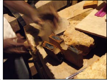
Figure 6-12: Broken Draw Trial with Black Core (Cohen 2010a)
