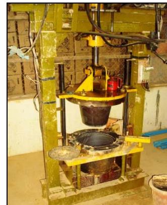
Figure 5-4: Filter Press with Cast-iron Mold, Cam-1 (IDECambodia 2009)
