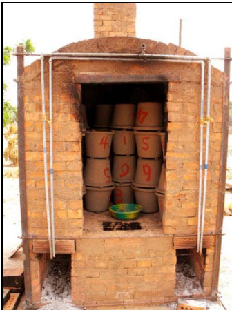
Figure 6-16: Flat Bottomed Filters Stacked in a Kiln (PotterswithoutBorders 2010)
