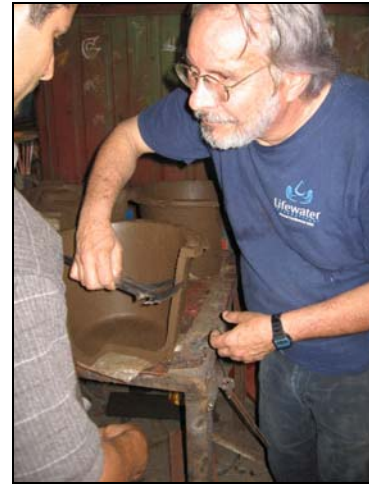
Figure 5-8: Checking Mold Alignment (Rayner 2006)
