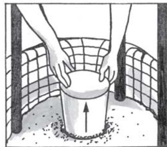
Pull the bucket partially out, leaving the stones in position. Fill the bucket again with stones and backfill with soil. Repeat for each layer.
