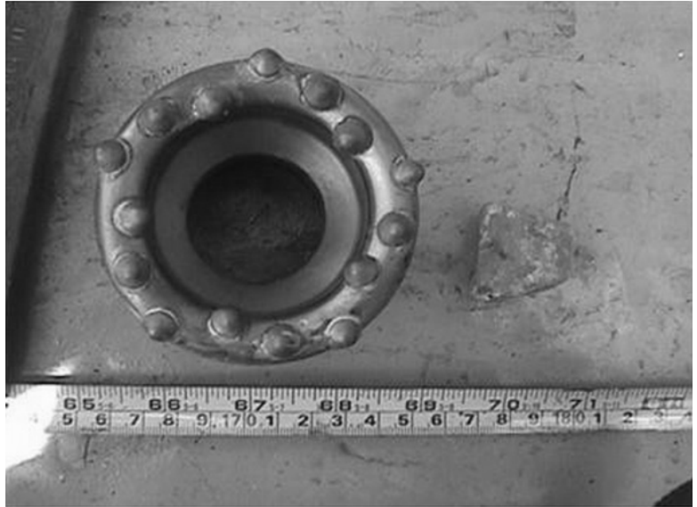
Figure 9. Hardened steel button bit
