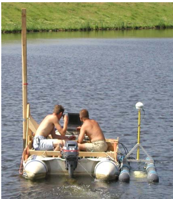
Figure 2: Minimal configuration used during the project to perform GeoRadar and seismic surveys parallel.
