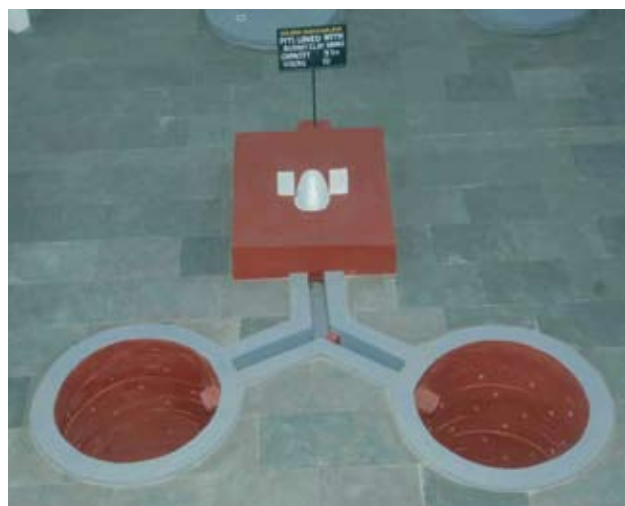
Figure 2. Sulabh twin-pit, pour-flush, compost toilet – a simple solution to achieve the Millennium Development Goal on sanitation
