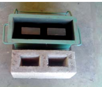
🔧 A hand mould to make sand/cement blocks.
