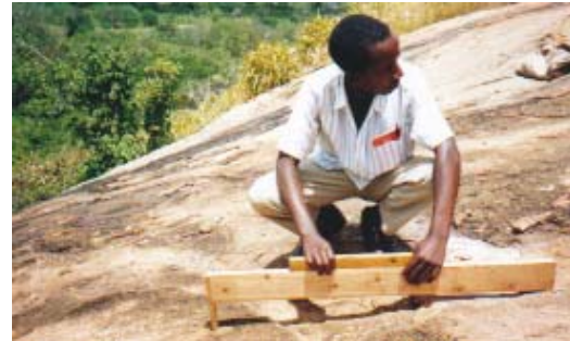
The gradient of a 3 cm slope per 100 cm is found by holding a spirit level horizontal on a 100 cm length of timber that has a leg being 3 cm long.
