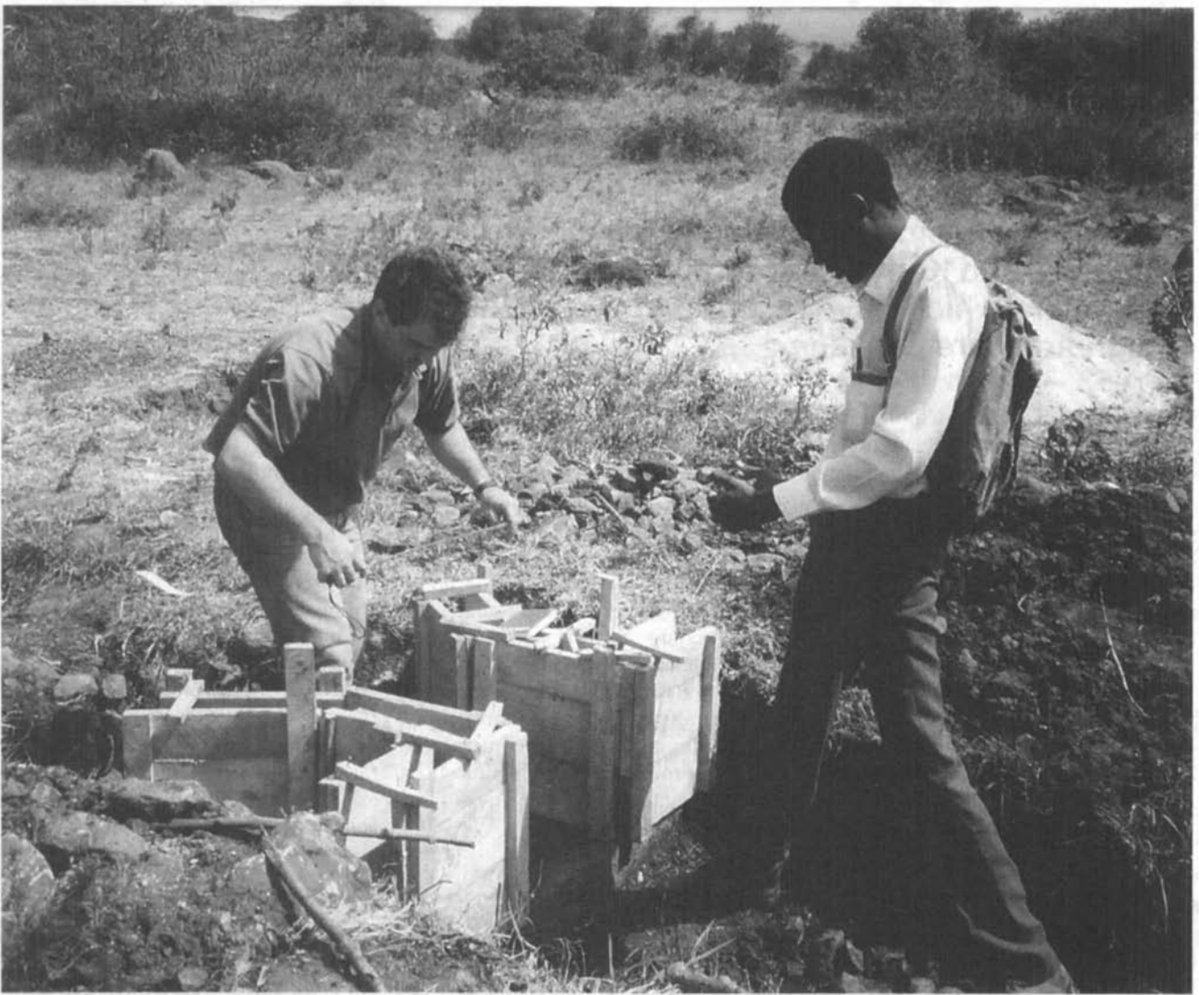
A flume is built to measure the flow in an unlined distribution channel in the Mutunyi irrigation scheme.
