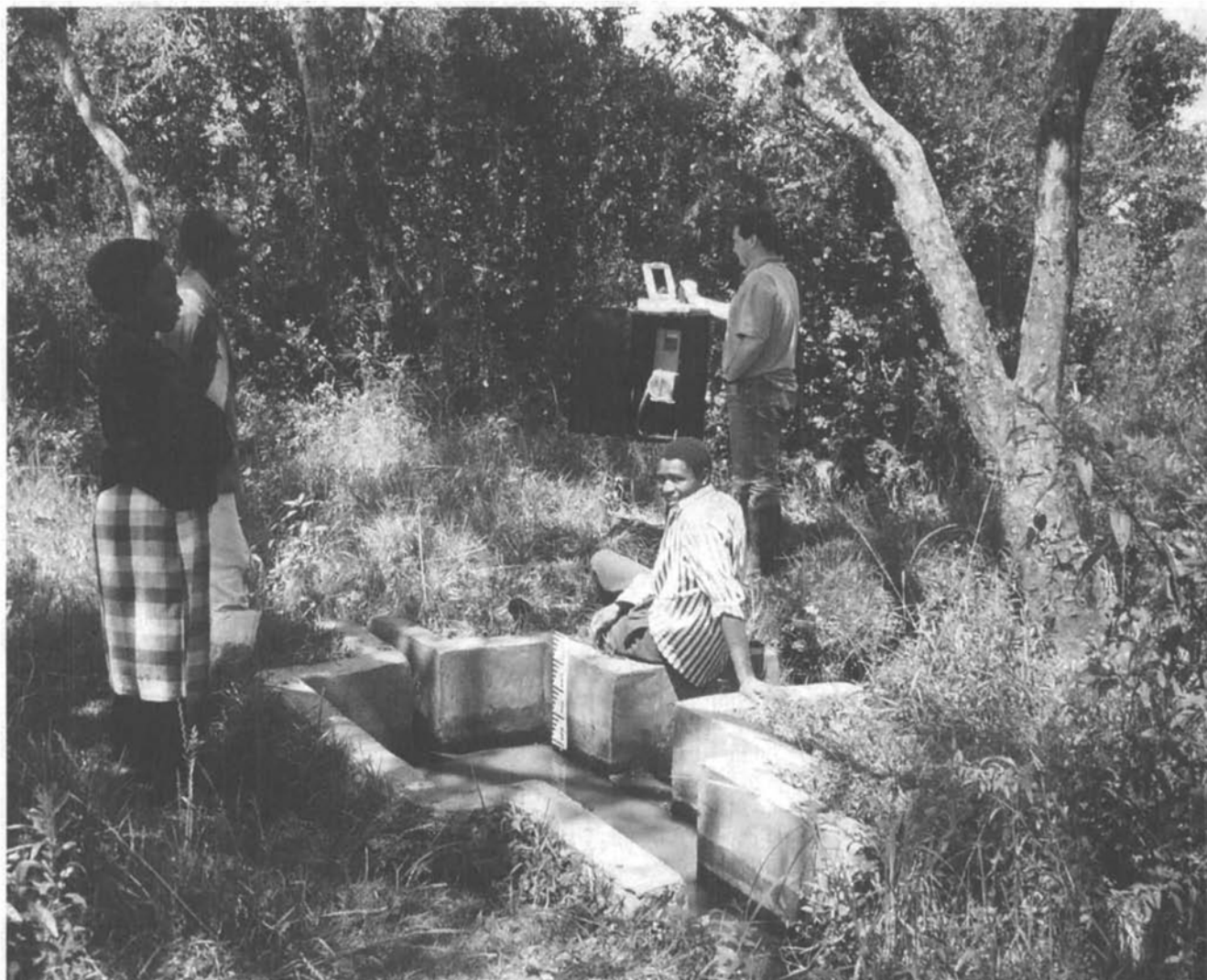
A data-logger is installed to measure the water flow at a division box at the Mathina irrigation scheme in Kenya.
