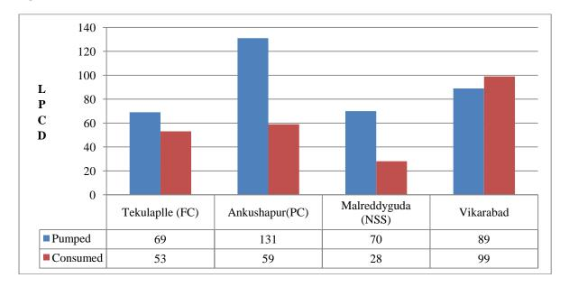
Figure 6: Unaccounted Water in the Test bed Areas
