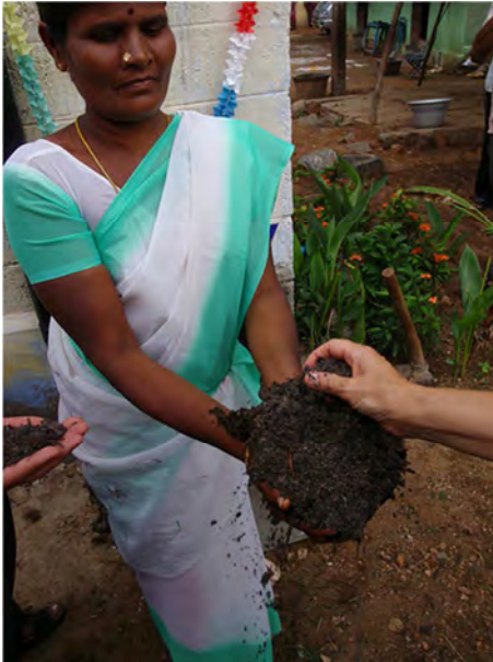
Figure 29. Dehydrated faeces from a UDDT in India. It contains no toilet papers as the users are `washers` (photo by J. Littmann). See also the opening of a vault here http://www.youtube.com/user/susanavideos#p/f/22/RRTPFs6JRX0
