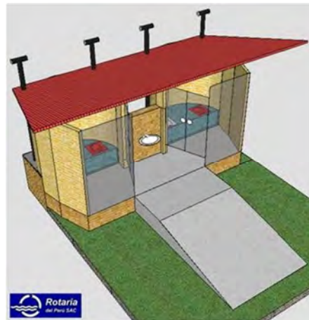
Figure 36 Drawing of a double vault bench UDDT with a ramp for a public toilet near Lima, Peru which could be easily modified with handrails and handlebars to make them accessible (photo by Rotaria del Peru SAC, 2010)
