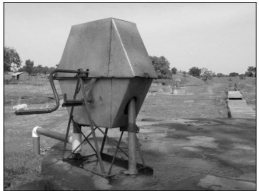
This heavy duty rope pump has greater protection
