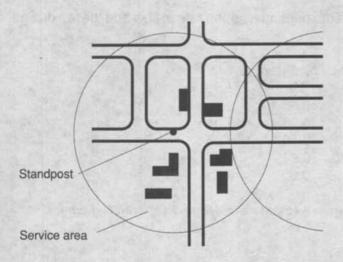
Good access is important both for users and maintenance. The standpost should be located centrally in the area it serves, ideally at a road junction, and must be on public land to avoid access problems. In hilly areas, remember it is easier to carry full containers downhill rather than uphill. Easy removal of waste water must also be considered.
