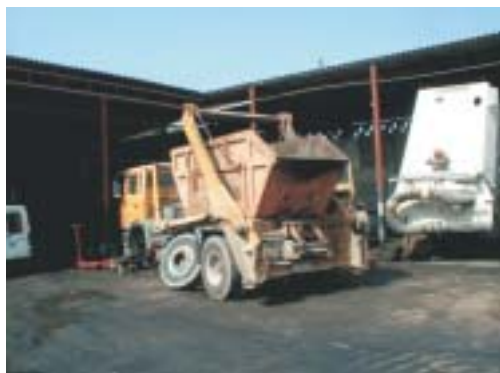
Skip-lift truck undergoing repair in a Palestinian workshop
