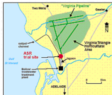
Figure 1. Location of the Bolivar ASR site, indicating the proximity to the Bolivar wastewater treatment plant and the horticultural area, where reclaimed water is used for irrigation
