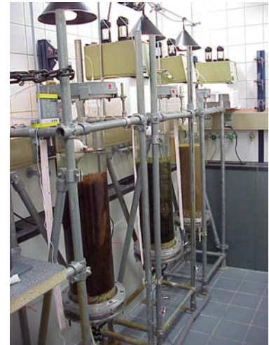
Figure 1. Filter columns in an air-conditioned room
