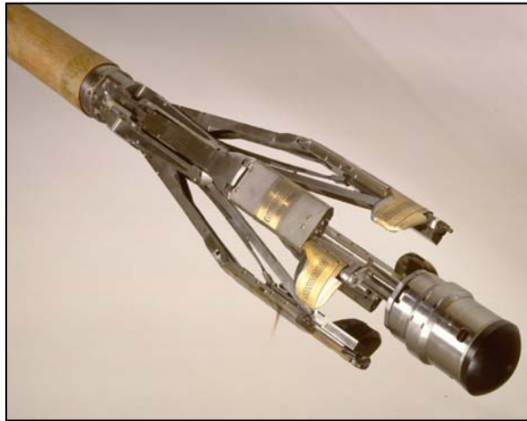
Figure 8. Measuring device for Formation Micro Imaging (FMI)
