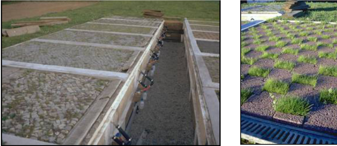
Fig. 1 and 2. Testing field of semi-permeable surfaces at the TU Berlin
