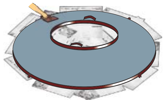
Figure 3-24: Fill the space between the two moulds with a mixture of 1:2 cement mortar and make it 2.5 centimetres thick and spread it uniformly.
