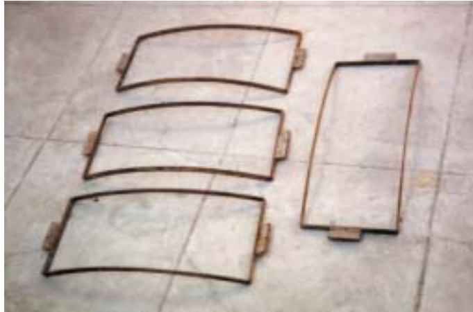
Figure 3-3: Iron segment moulds for casting tank segments.
