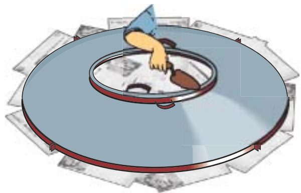
Figure 3-27: Place the 80 centimetres diameter inner mould on top of the paper-covered sand base to cast the tank mouth. Fill the space between the two moulds with the 1:2 cement mortar and fill up to the top level of the moulds.
