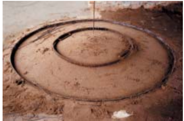
Figure 3-21: Prepare a conical sand base inside the lower cover outer mould (diameter 162 centimetres) with a height of 18 centimetres at the centre. Insert a piece of wire to mark the centre.
