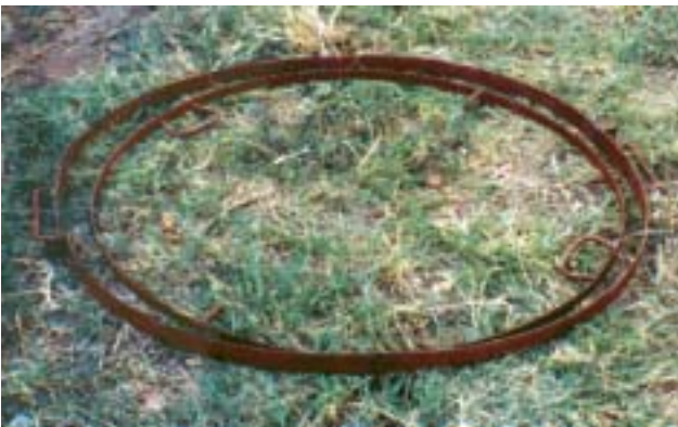
Figure 3-4: Measurements of moulds (set of 2) for the UPPER COVER of the tank. Iron strips 0.4 centimetre thick and width of 6 centimetres and 3 centimetres are used to make the moulds. Diameters of the outer and inner moulds are 100 centimetres and 92 centimetres, respectively. Details of dimensions are shown in the drawing.
