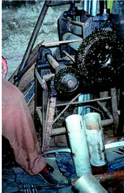
Manufacturing of treadle pump cylinders.
