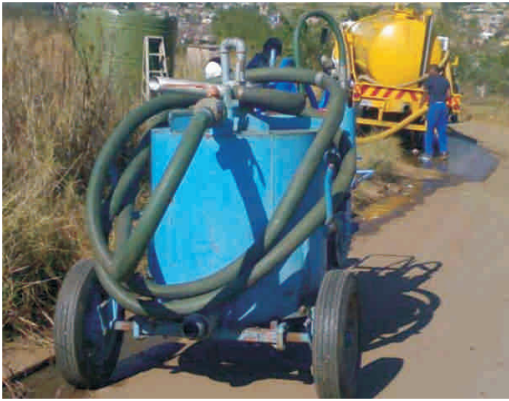
Figure 30 : Vacutug being trialled in Pietermaritzburg
