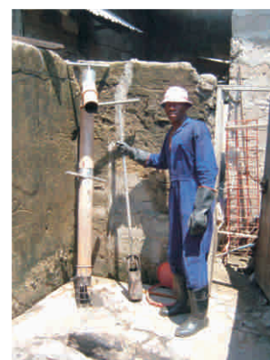
Figure 18 : The 'gulper', being field tested in Tanzania
