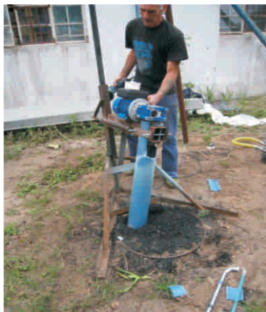
Figure 28 : Early prototype of a Pit Screw Auger (PSA)
