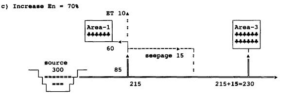
Figure IV Impact of Increasing Efficiency En (iv) Return flows are reused by downstream user Area-3
