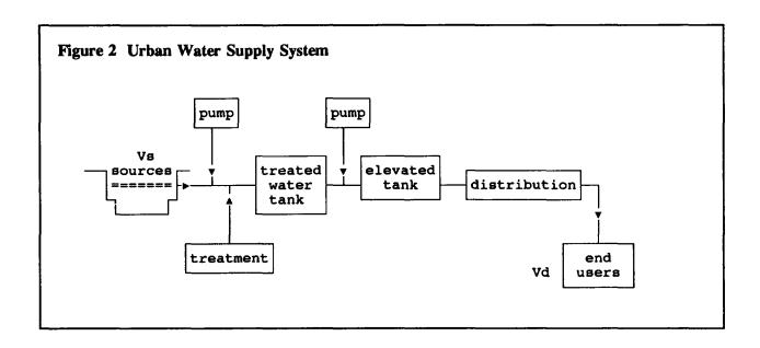
In urban water supply projects, one common measure of Ed is through use of an indicator called *unaccounted-for* water (UFW), i.e. UFW = Vs - Vd (see Figure 3), therefore,
