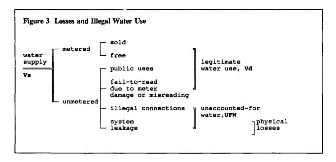
where: UFWr = UFW/Vs, standing for the ratio of unaccounted-for water.
