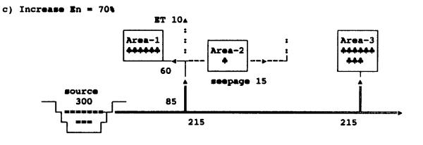
Figure II Impact of Increasing Efficiency En (ii) Return flows are reused by Area-2 only
