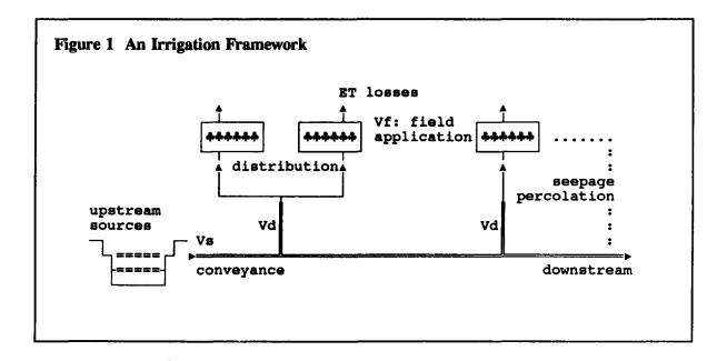
i. Conveyance is the movement of water from its sources (reservoirs, river diversions, wells or pumping stations) through main and secondary canals to the tertiary offtake of a distribution system. Conveyance efficiency, Ec, is defined as:
