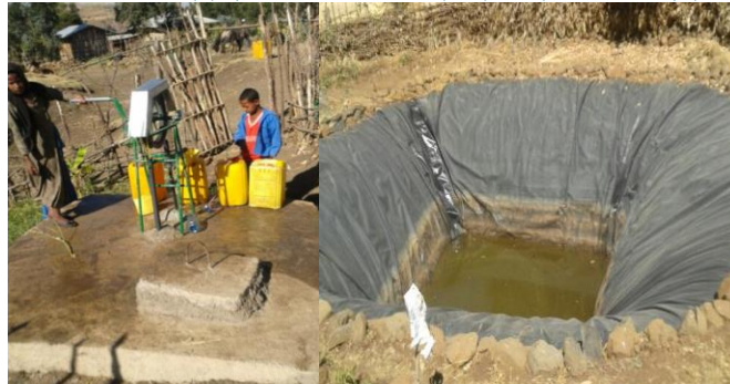
Photo 7: Self-supply in Kelala, a) rope pump, b) family pond
