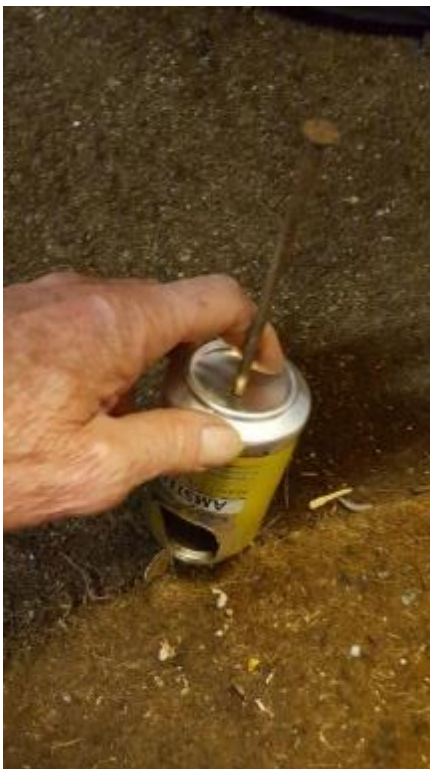
Make a hole in the bottom with a nail.
