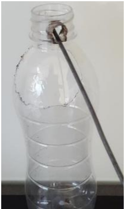
Make a hole of 10 mm in the top (strong) part of the bottle
