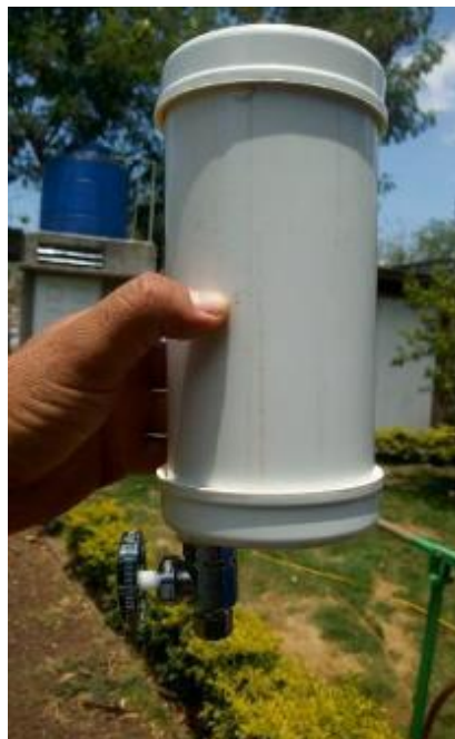
Soap dispenser. Made of a PVC pipe (2 or 3 inch), 1 or 2 end caps and a faucet (tap).
