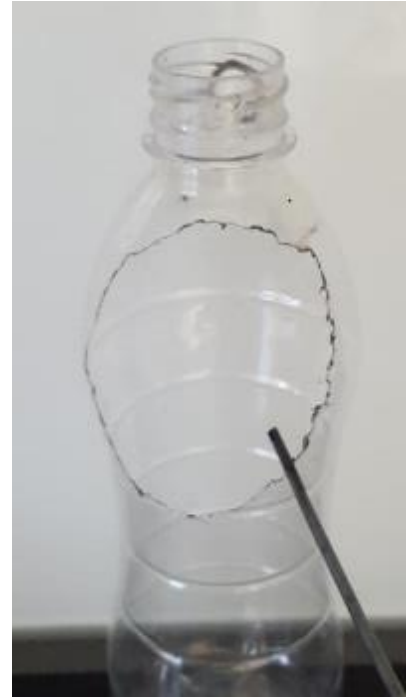
Make a hole of around 5 cm (2 inch) with the hot wire or a knife
