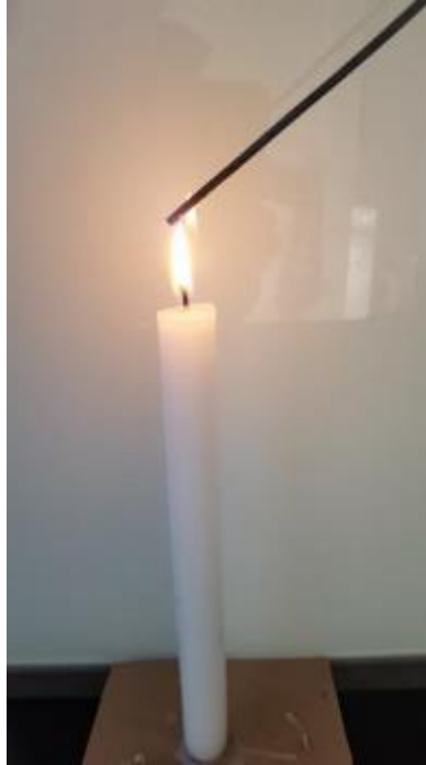
Holes in a plastic Dip Tap can be made with a hot wire, heated with a candle or other fire
