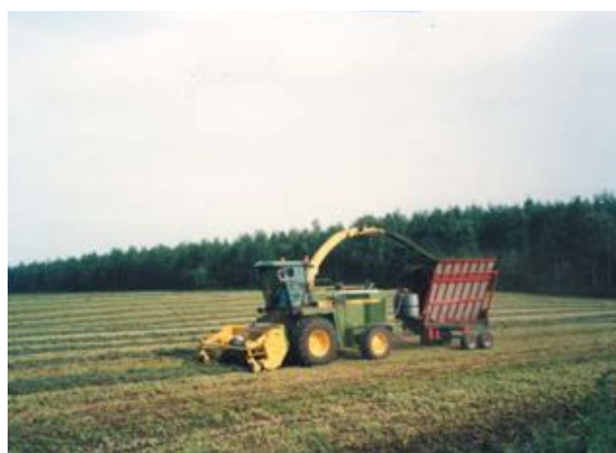
Harvesting pasture plants by a self-propelled harvester and loading chopped plants to a transporting car
