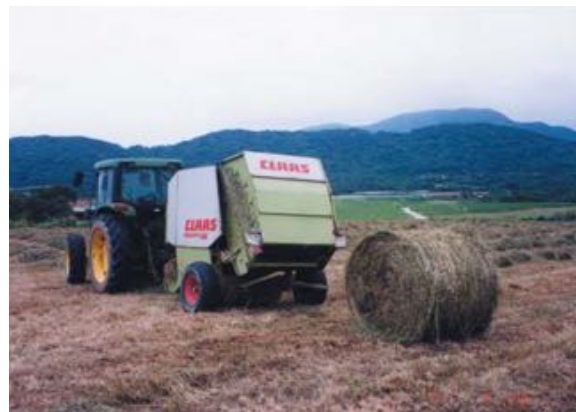
A pasture plant roll bale made by a roll baler
