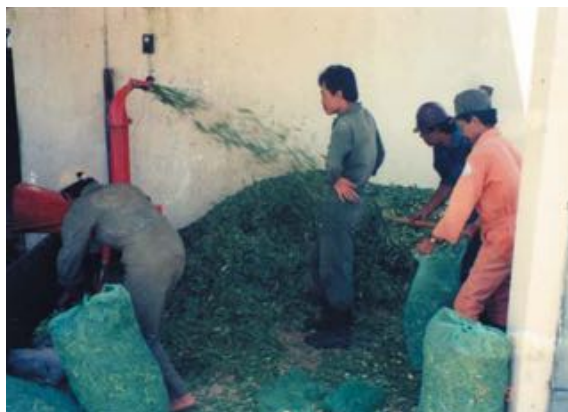
Chopping of raw materials (Elephant grass) by a small-sized cutter with an engine
