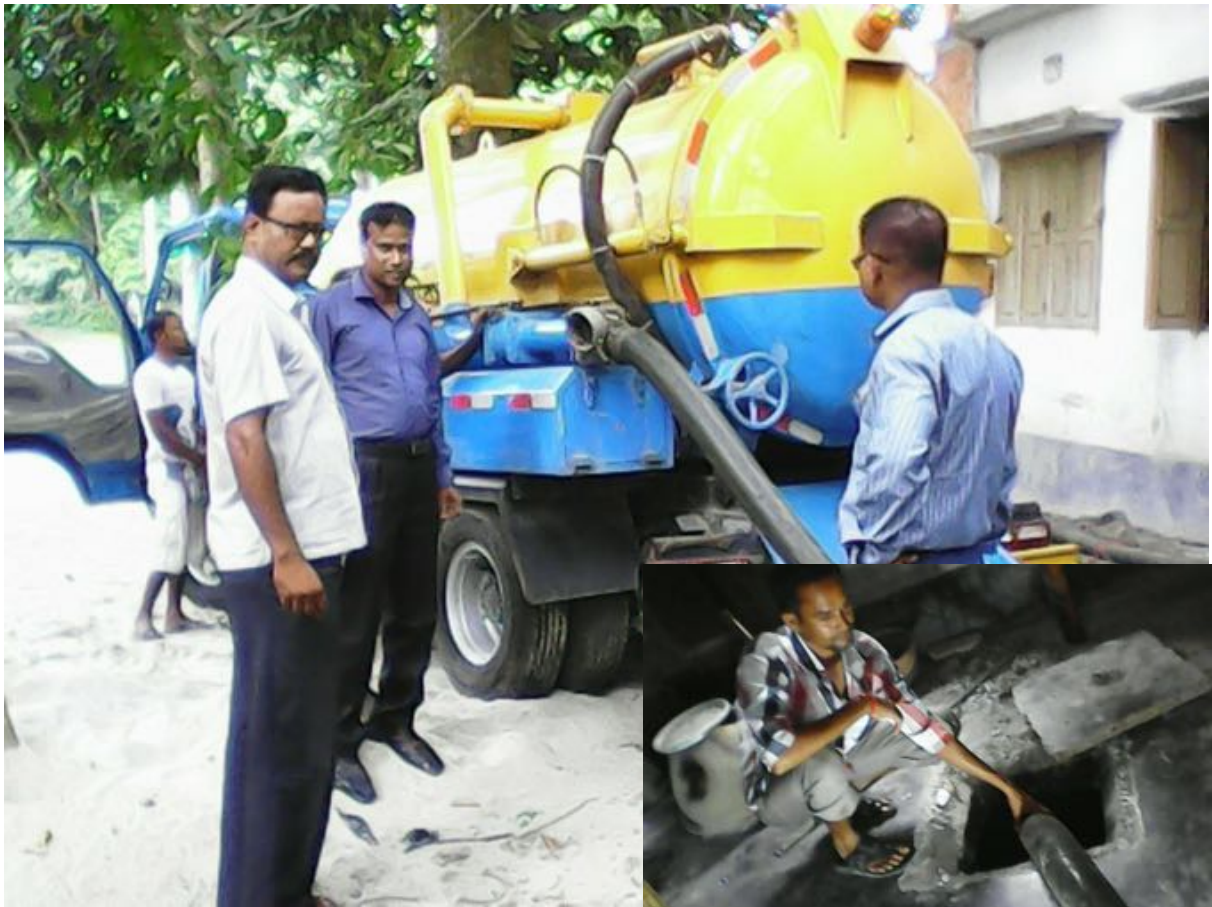
Truck Mounted Vacutug (inset Emptying Safety Tank)
